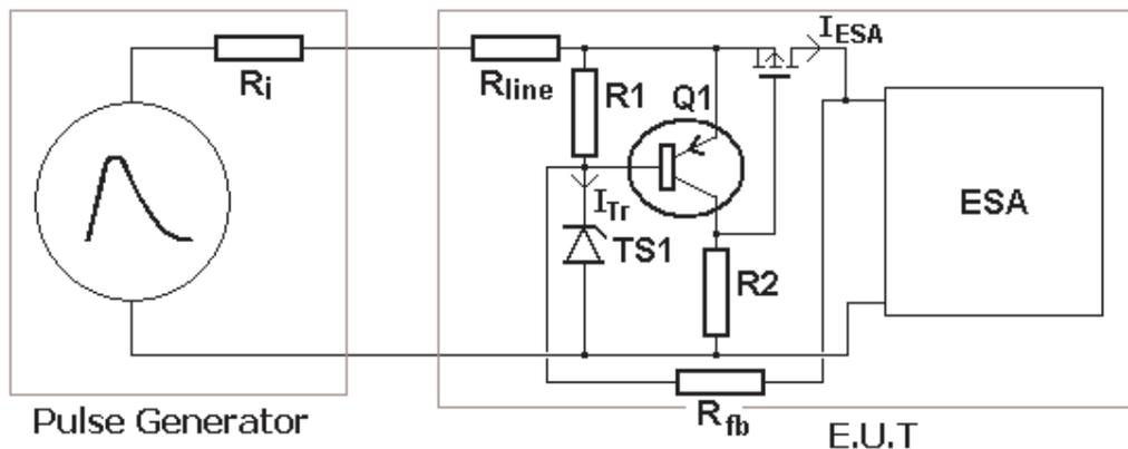
Figure 9 – P-FET Isolation Switch Example Circuit
