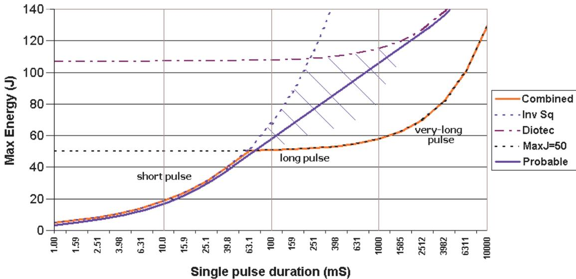
Figure 6 – 5KP-Series Calculated Energy Limit -v- Pulse Duration
