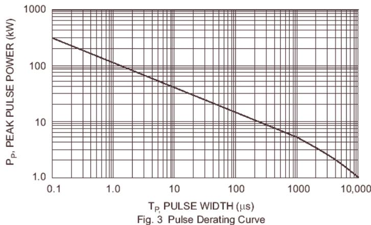
Figure 5 – WTE 5KP-Series Pulse Width Derating Curve<sup>[3]</sup>
