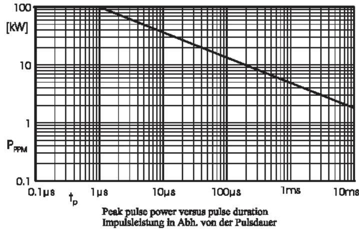
Figure 4 – Diotec 5KP-Series Pulse Width Derating Curve<sup>[2]</sup>
