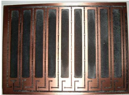
Paper transferred board prior to etching
