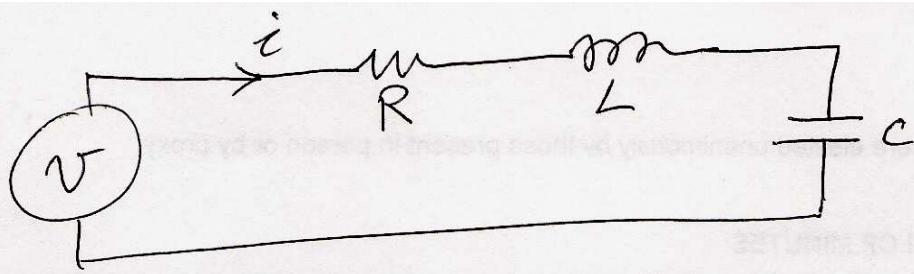
$$iR + L \frac{di}{dt} + \frac{1}{C} \int i dt = V \cos(\omega t + \phi) \quad (1)$$
