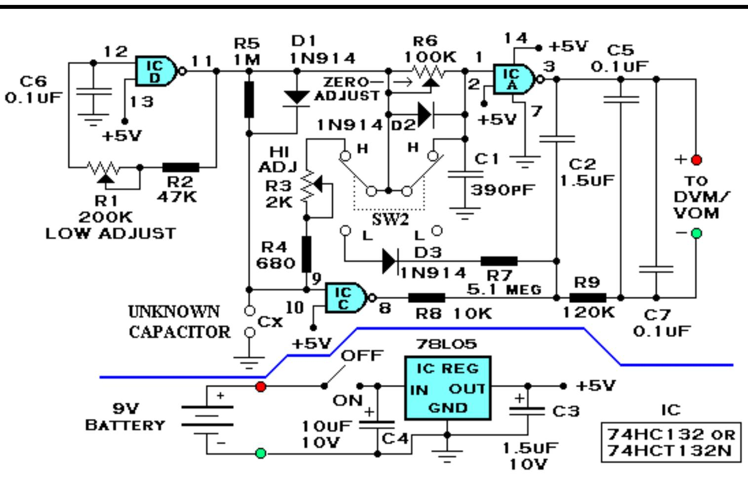
*All components are 10% tolerance. An LM7805 may be substituted for the 78L05. All fixed resistors are 1/4 watt carbon composition. Capacitors are in uF unless otherwise indicated.*
