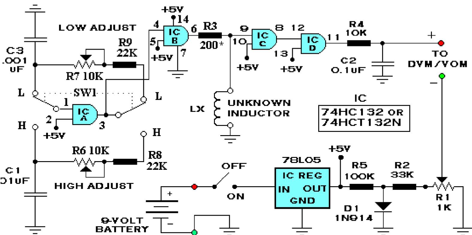
*All components are 10% tolerance. 1N4146 or equivalent may be substituted for D1. An LM7805 may be substituted for the 78L05. All fixed resistors are 1/4 watt carbon composition. Capacitors are in  $\mu\text{F}$ . R3 value may need to be increased or decreased slightly if calibration cannot be achieved as described in text.*
