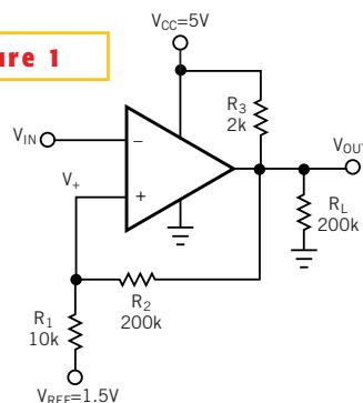
**$R_1$  and  $R_2$  add hysteresis to the comparator to prevent multiple switching.**
