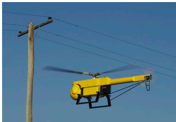
Fig. 1. CSIRO / UAV Vision mini-helicopter flying close to a power line to demonstrate its potential inspection capability.
