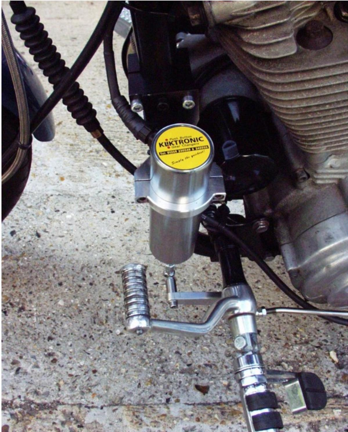
A 'Kuryakyn Magnum Quick Clamp' of the appropriate size for the frame downtube will give a support for our swivel clamp. You will see that in order to achieve the correct angle (90 Degrees) and length of stroke (1") we have bolted an additional lever to the original.
