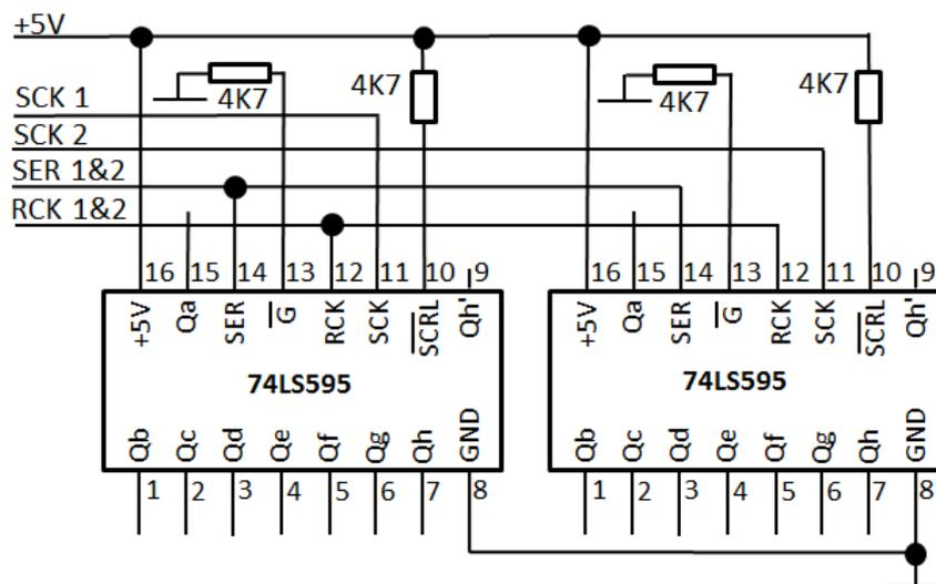
This function block is ideal when using the 74LS595 to drive a 7-segment display. Use it together with FB107, which is a pattern-lookup function block.
