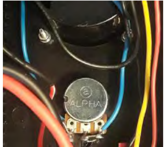
Figure 11 - Zero-adjust Potentiometer Meter Connection
