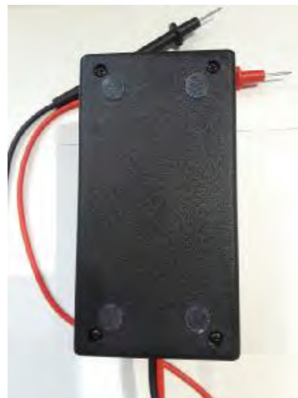
Figure 12 - Rubber Bumper "Feet" Installed
