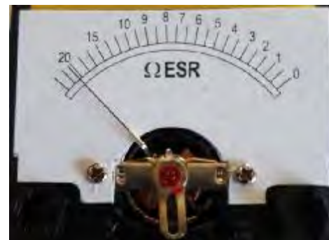
Figure 14 - Meter Faceplate Mounting
