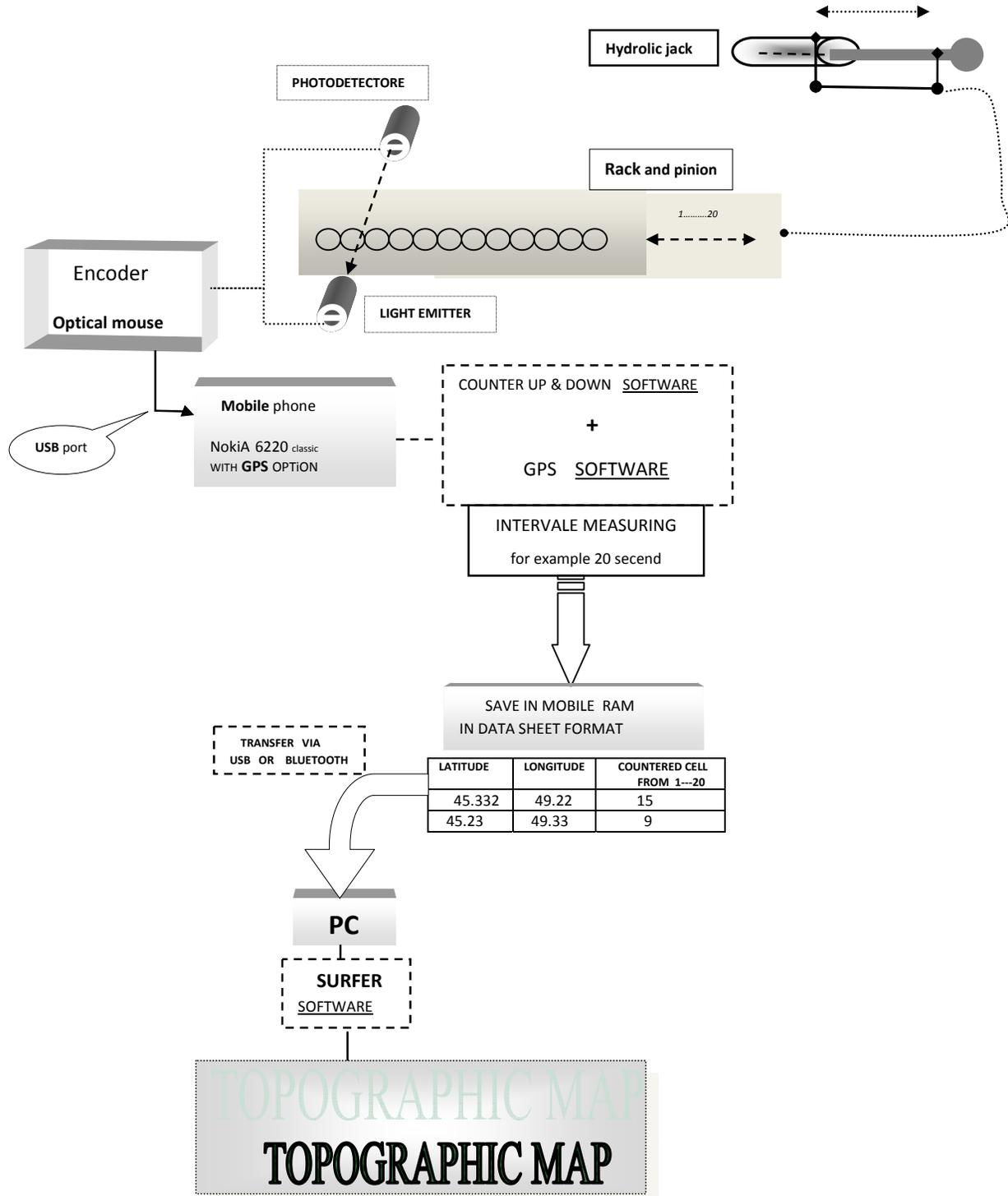
please note that the mobile phone is installed at the place of the measuring such as the yard of company or field but the pc is located at the office. actually the data will be saved at the mobile phone Ram then it will be transferd into the pc which is far away at the office ./
