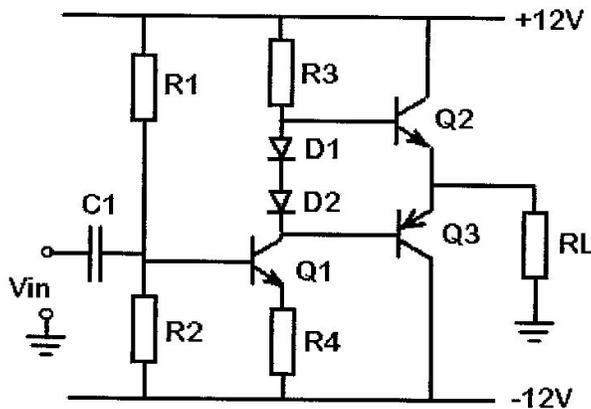
Let  $R_1 = 22k$ ,  $R_2 = 2.2k$ ,  $R_3 = 1.5k$ ,  $R_4 = 120\Omega$  and  $C_1 = 1\mu F$ . (110 marks)
