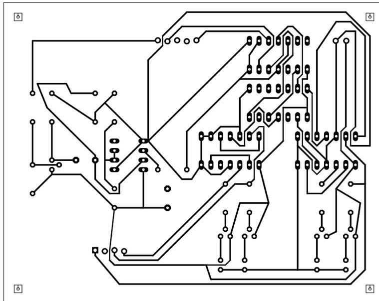
OUTPUT SECTION\_SOLDER SIDE
