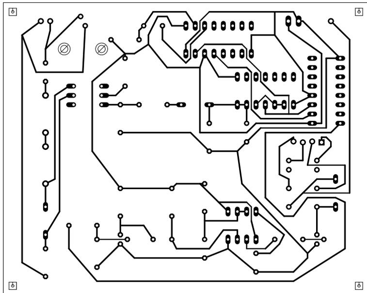
RING DETECTION SECTION\_SOLDER SIDE
