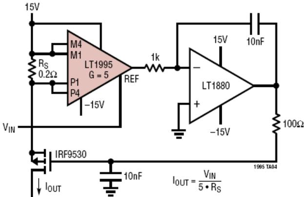
The LT1995 amplifies the sense resistor drop by 5V/V and subtracts that from  $V_{IN}$ , providing an error signal to an LT1880 integrator. The integrated error drives the PMOSFET as required to deliver the commanded current.
