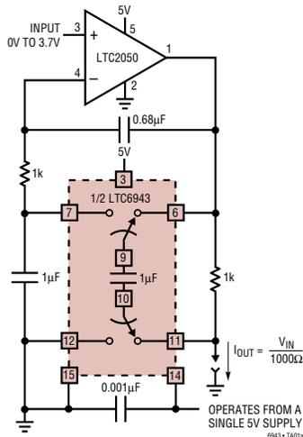
The LTC6943 is used to accurately sample the voltage across the 1kΩ sense resistor and translate it to a ground reference by charge balancing in the 1μF capacitors. The LTC2050 integrates the difference between the sense voltage and the input command voltage to drive the proper current into load.
