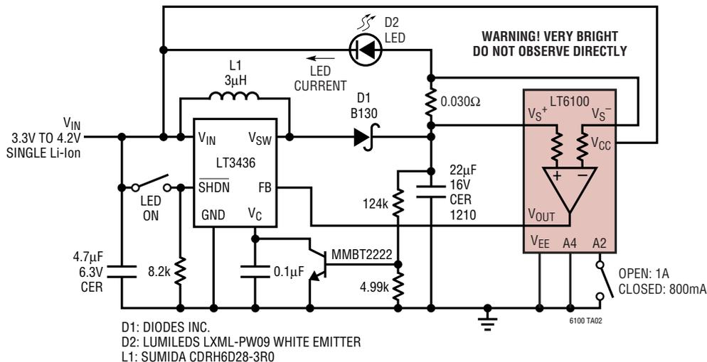
The LT6100 is configured for a gain of either 40V/V or 50V/V depending on whether the switch between A2 and V<sub>EE</sub> is closed or not. When the switch is open (LT6100 gain of 40V/V), 1A is delivered to the LED. When the switch is closed (LT6100 gain of 50V/V), 800mA is deliv-
