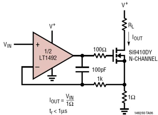
This is a simple controlled current sink, where the op amp drives the NMOSFET gate to develop a match between the 1Ω sense resistor drop and the  $V_{IN}$  current command. Since the common-mode voltage seen by the op amp is near ground potential, a “single-supply” or Rail-to-Rail type is required in this application.
