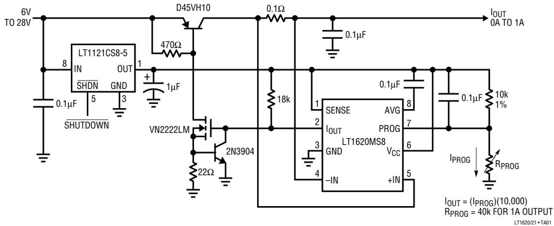
The current output can be controlled by a variable resistor ( $R_{PROG}$ ) connected from the PROG pin to ground on the LT1620. The LT1121 is a low-dropout regulator that keeps the voltage constant for the LT1620. Applying a
