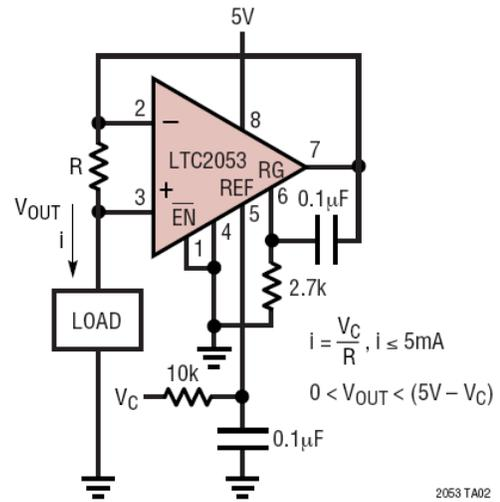
The ultra-precise LTC2053 instrumentation amplifier is configured to servo the voltage drop on sense resistor R to match the command  $V_C$ . The LTC2053 output capability limits this basic configuration to low current applications.
