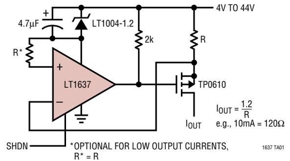
This is a simple current-source configuration where the op amp servos to establish a match between the drop on the sense resistor and that of the 1.2V reference. This particular op amp includes a shutdown feature so the current source function can be switched off with a logic command. The 2kΩ pull-up resistor assures the output MOSFET is off when the op amp is in shutdown mode.
