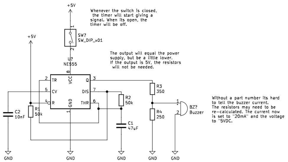
Capacitors should be as close as possible to IC.
