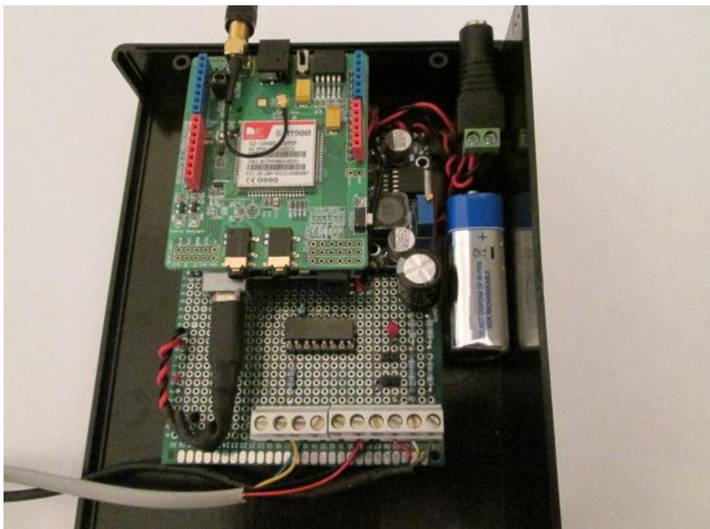
The these few pages give a general view of the complete project for this diy Arduino based sms controller.
