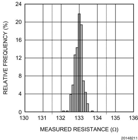
**FIGURE 4. Typical Resistor Variation: 1% General Purpose 0805 SMD**
