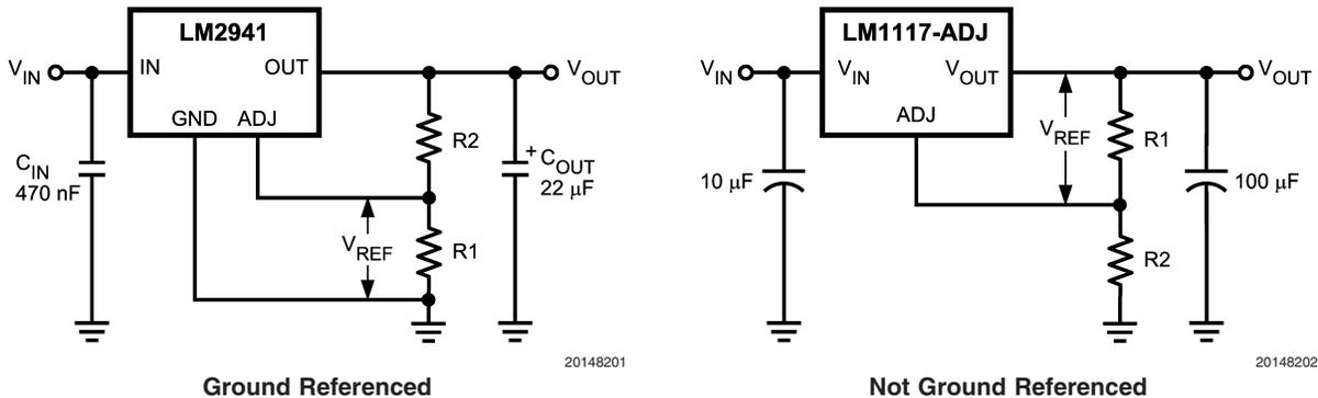
FIGURE 1. Adjustable Regulators: Common Topologies
