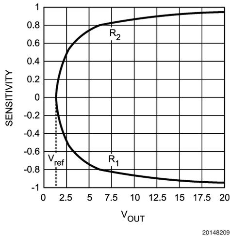
FIGURE 2. – Sensitivity to Resistor Variations vs.  $V_{out}$
