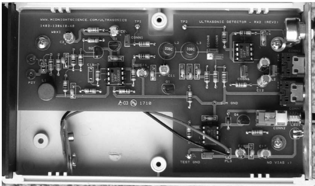
Figure 7 —The AGC circuit is incorporated into the circuit board for the Ultra-RX2 ultrasonic receiver. The AGC circuit is in the top left corner of the circuit board. Note that the component designators on the board may not match the designators on the schematic of Figure 6.
