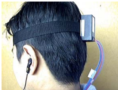
(b) Gyroscope sensor for head tracking.
