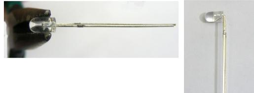
2. Insert the LED into the holes on the board. Align the negative (-) lead with the negative pad. Solder the leads now or cut to board thickness then solder.
