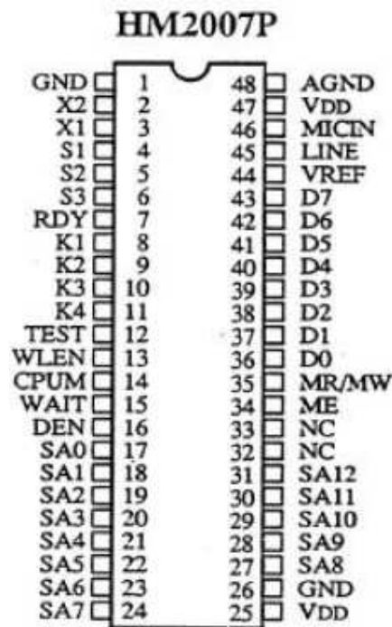
Figure 3.3: Pin layout of the HM2007 Dip package.
