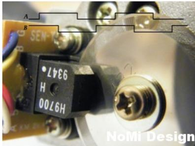
This bit will decode a quadrature input from a rotary incremental or linear position sensor, it polls two inputs (PIND4 & PIND5) to convert the incoming grey code into respective direction and count, tallying the position in a signed 16bit variable. It can be run on pinchange interrupt, timer interrupt, or called as a function. It also contains a provision for missed transitions.
