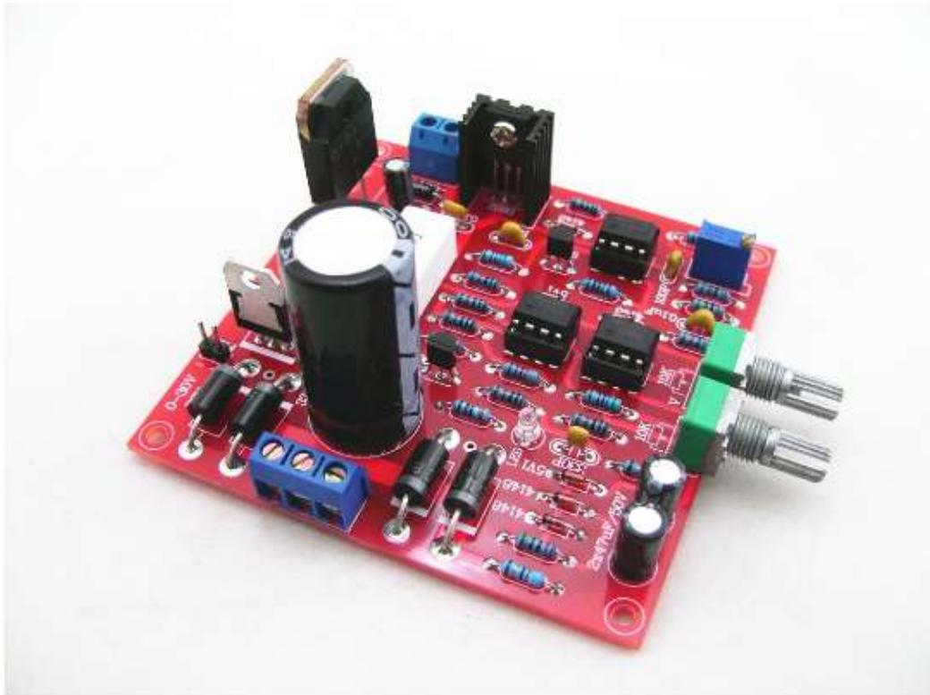
Potentiometer can install on the board directly,can install on breadboard by using socket and wire.it can also change a Multi-turn potentiometer which make adjustable finer.
