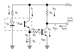
HOA1874-11 Parameters:  $I_L$  = .3 mA min. @  $I_F$  = 20 mA,  $V_{CE}$  = 5 V  $V_F$  = 1.6 V max. @  $I_F$  = 20 mA Q1 is a 2N2222 (HFE = 60 min.)  $V_{CC} = 5.0 V$  nominal
