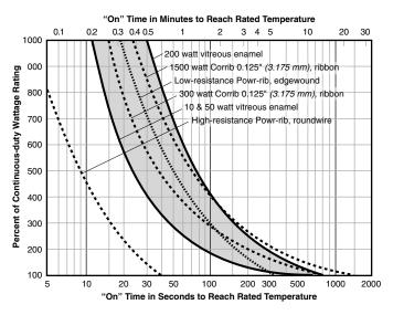
Fig. 9: Time Required for Typical Resistors to Reach Rated Operating Temperatures at Various Watt Loads.
