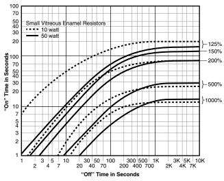
Fig. 10: 10 Percent of Continuous Duty Rating for Pulse Operation of small to Medium Size Vitreous Enameled Resistors.
