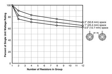
Fig.6: Derating of Resistors to Allow for Grouping
