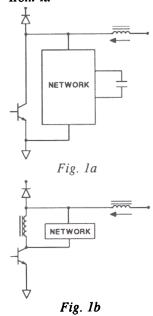
All of the other classifications of snubbers relate to the ways in which the energy is transferred to and from the snubber. If the energy stored in the snubber is dissipated in a resistor the snubber is classed as dissipative but if the energy is moved back to the input or ahead to the output the snubber is classed as non-dissipative even though there may be some small losses. A snubber is classed as polarized or non-polarized depending on
