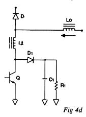
Where I is the maximum peak switch current,  $\Delta V$  is the peak voltage the capacitor will charge to,  $\Delta t$  is the rise time of the voltage and C is the value of the capacitor. The resistor is then chosen to have a time constant which is small compared to the switching period. A typical value for the time constant would be one tenth of the switch maximum on time.
