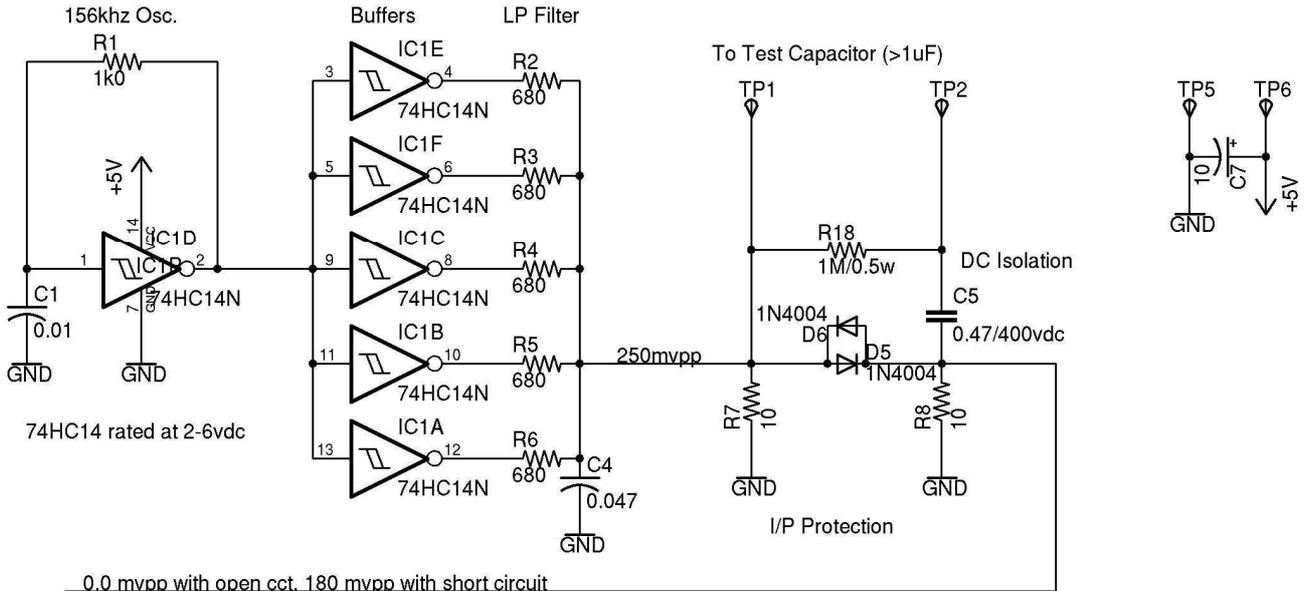
Threshold of rectifier diodes is used create an expanded scale AC voltmeter.
