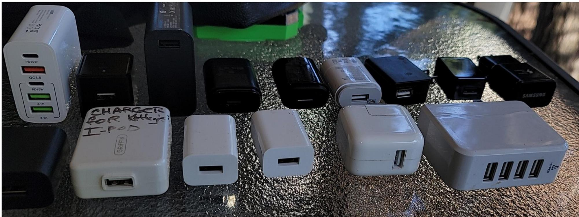
A random assortment of 15 USB chargers were tested to determine the AC leakage characteristics, and the larger application to SMPSs.
