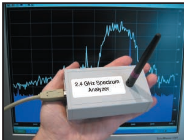
Photo 1 —The spectrum analyzer consists of a small RF receiver circuit connected to a PC via a USB port. A custom Windows software application controls the hardware and displays the spectrum.
