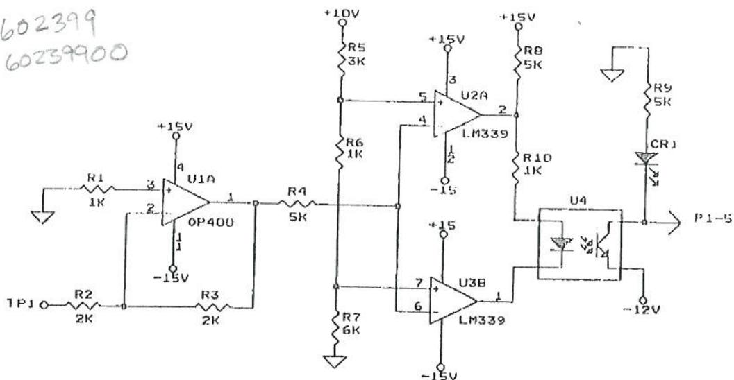
A component has failed in the preceding circuit. If the voltage at TPI is too negative, CR1 turns off as designed. The problem is that CR1 is on when TPI is at 0 volts. Which component has failed?
