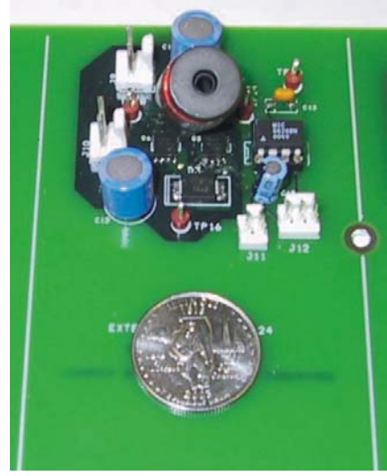
Fig. 3: Photograph of 3 W (nominal) low-input-voltage converter.
