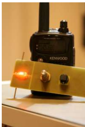
Picture of the RF field monitor in front of a handheld transceiver. For this picture, I short-circuited the pushbutton. Since this monitor is DC powered, the lamp keeps glowing after the transceiver is returned to receive mode. (click to enlarge).
