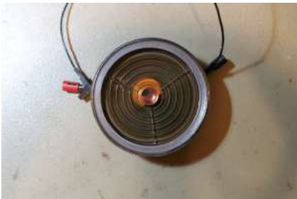
A SI-8B (CH-8B) Geiger tube connected to a suitable power supply as specified in its datasheet: 390 V with a 4.7 M \Omega series resistor. (click to enlarge).
