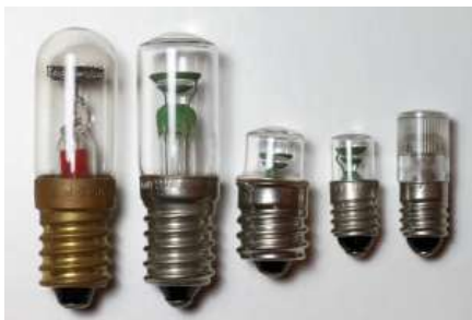
Five glow lamps with screw mount intended for mains indicator light applications: the three on the left have an E14 socket and the two on the right E10. They all have an integrated ballast resistor and are all suitable for direct connection to a 230 V AC mains. (click to enlarge).
