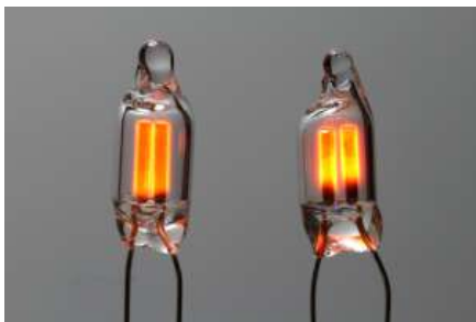
Two brand new and identical lamps (same production lot) driven in the same conditions (same power supply and ballast resistor value) can glow very differently. (click to enlarge).
