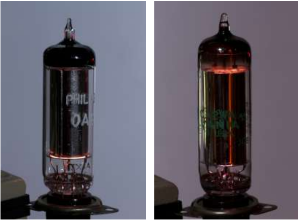
Picture of two 0A2 voltage stabilizer tubes rated for 150 V. On the left a tube manufactured by Philips and on the right a tube manufactured by Sylvania. Both tubes are on, but only little light leaks out. (click to enlarge).
