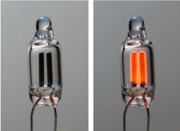
Close-up of a common NE-2 like neon glow lamp, "off" on the left and "on" on the right. (click to enlarge).
