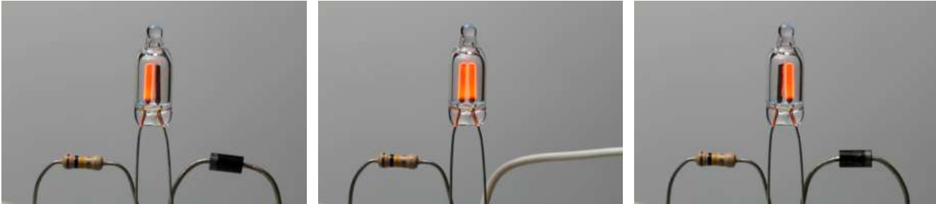
Pictures of the same neon glow lamp with the negative electrode on the left (left), with AC (center) and with the negative electrode on the right (right). Please observe the orientation and presence of the diode. (click to enlarge).
