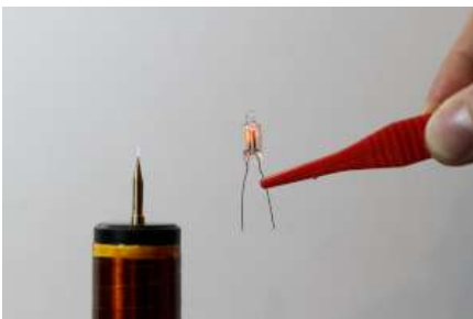
Picture of a neon glow lamp in a strong electromagnetic field. Please remark that the lamp held with insulating tweezers. (click to enlarge).
