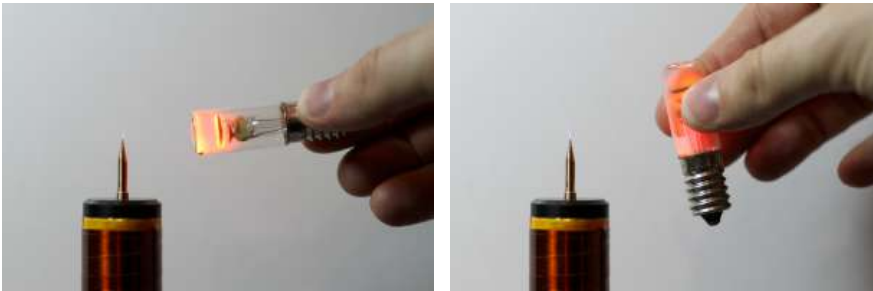
Picture of a neon glow lamp in a strong electromagnetic field. Please remark that the lamp is not connected and that it glows even when I'm holding it by the glass. (click to enlarge).
