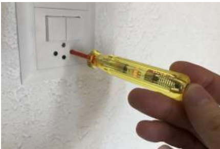
Picture of a mains test screwdriver in action. Note how the user touches the back ring to close the circuit. (click to enlarge).
