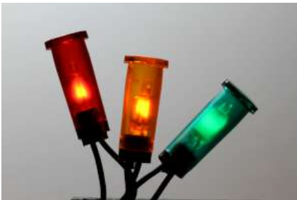
Three mains voltage indicator lamps with integrated ballast resistor. The red and orange lamps use a true neon glow lamp while the green one is of the fluorescent type. (click to enlarge).
