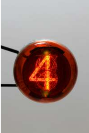
Picture of a Philips Z520M nixie tube with the "4" shaped cathode connected to the circuit. (click to enlarge).
