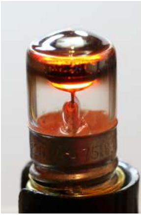
Picture of a glowing lamp after several years of service: it still glows but the glass is blackened by the metal sputtered off the electrodes. (click to enlarge).
