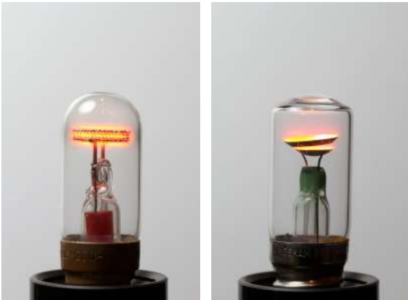
Pictures of two similar neon glow lamps. The lamp on the left has bare electrodes and the glow is all around them. The lamp on the right has the bottom part of the electrodes painted with an insulating material: only the top part glows. (click to enlarge).
