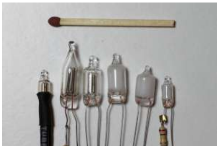
Six full glass glow lamps. From left to right: a miniature neon glow lamp Ø 4 mm × 8 mm, a true General Electric NE-2 neon glow lamp Ø 6.35 mm × 27 mm, a common neon glow lamp Ø 6 mm × 19 mm, a green fluorescent glow lamp, a blue fluorescent glow lamp and a miniature green fluorescent glow lamp. (click to enlarge).
