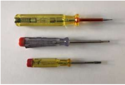
Picture of three mains tester screwdrivers. The bottom one is an old one and its shaft is not insulated. (click to enlarge).
