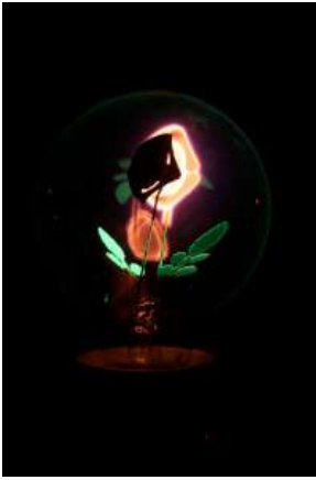
Picture of a rose decorative lamp when DC powered. Please remark that only one electrode glows pink, but both leaves glow green. (click to enlarge).
