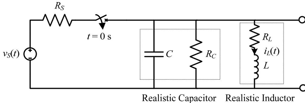
we will define the “output” of this *RLC* network as the current through the realistic inductor,  $i_L(t)$ , and the “input” is the voltage source,  $v_S(t)$ .
