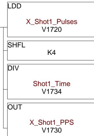
Calculate the B axis speed for the first shot.
