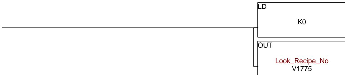
Upon a command from the HMI to look at recipe data, calculate the pointer to the memory location for the data.
