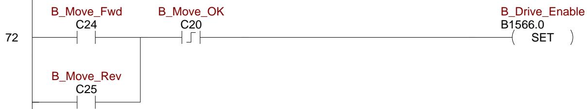
If the command is to move forward turn the the CTRIO direction output.
