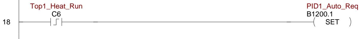
When the PID loop is in auto mode (running), load the setpoint and feedback into the control registers.
