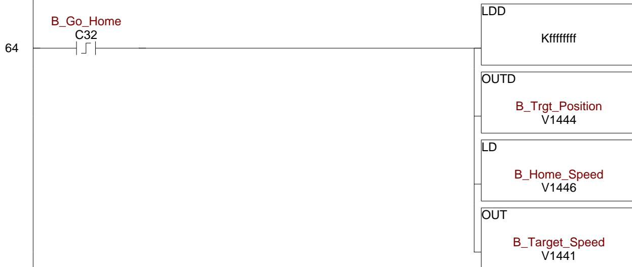
When moving to dispense, use the calculated values for the frequency and target position.
