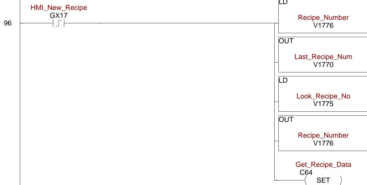
Upon a command to fetch recipe data, calculate the pointer to the memory location for the data.
