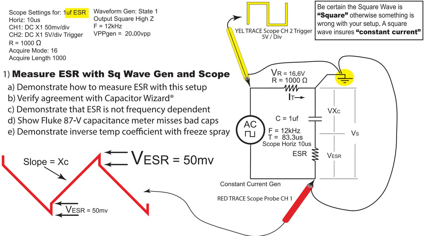
Adjust the scope horiz and vertical & waveform gen until a pattern such as above is observed.
