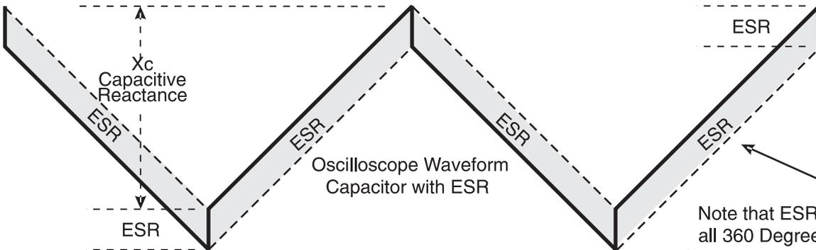
Note that ESR exists through all 360 Degrees. That means POWER is being dissipated through the entire 360 Degrees.  $P = I^2 * ESR$
