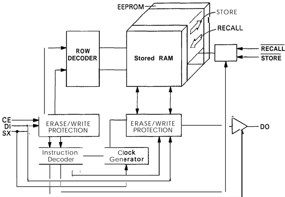
**Figure A-1 O. ER59256 Block Diagram**
