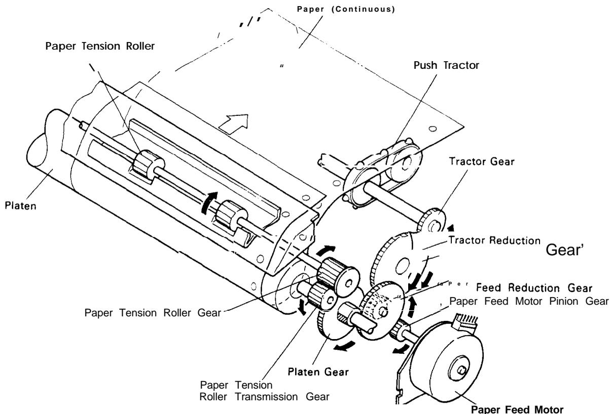
Figure 2-39. Push Tractor Feed Operation
