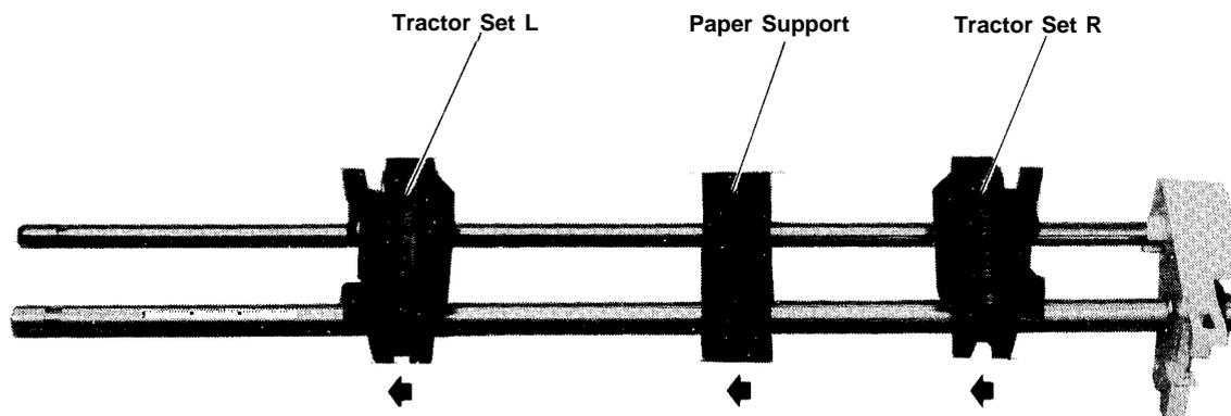
Figure 4-37. Extraction of Tractor Set L, Paper Support, and Tractor Set R
