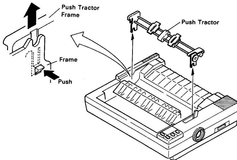
Figure 4-4. Push Tractor Removal
