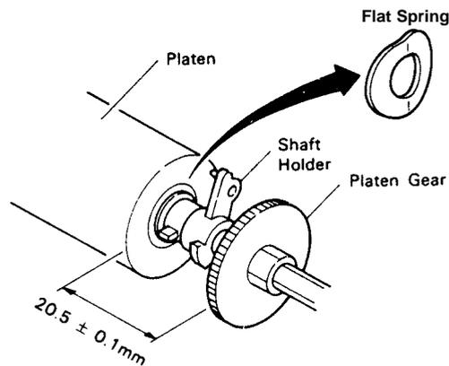
Figure 4-26. Platen Unit Reassembly
