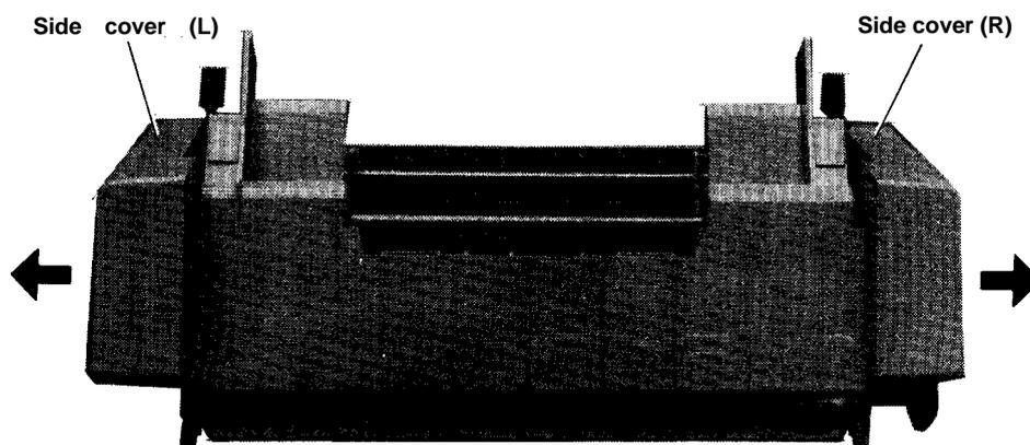
Figure 3-5. Side Cover Removal
