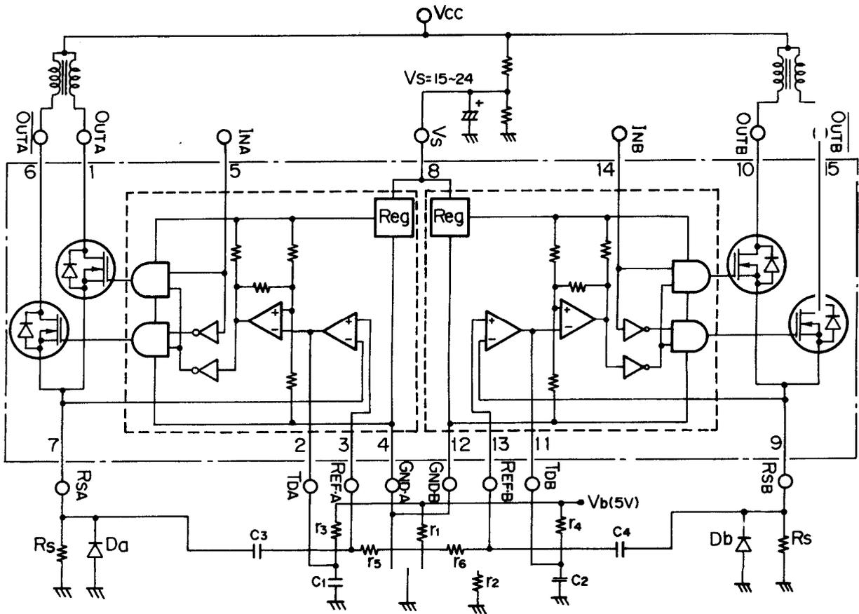
**Figure A-1 2. SLA7020M Functional Equivalent Circuit**
