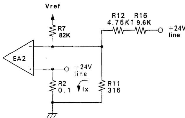
**Figure 2-18, Over-Current Protection Circuit**
