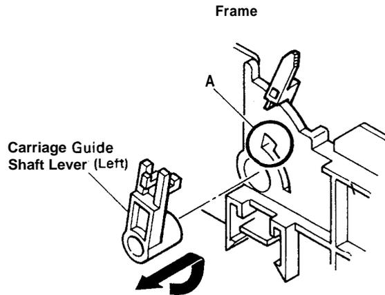
Figure 4-29. Removal of Carriage Guide Shaft
