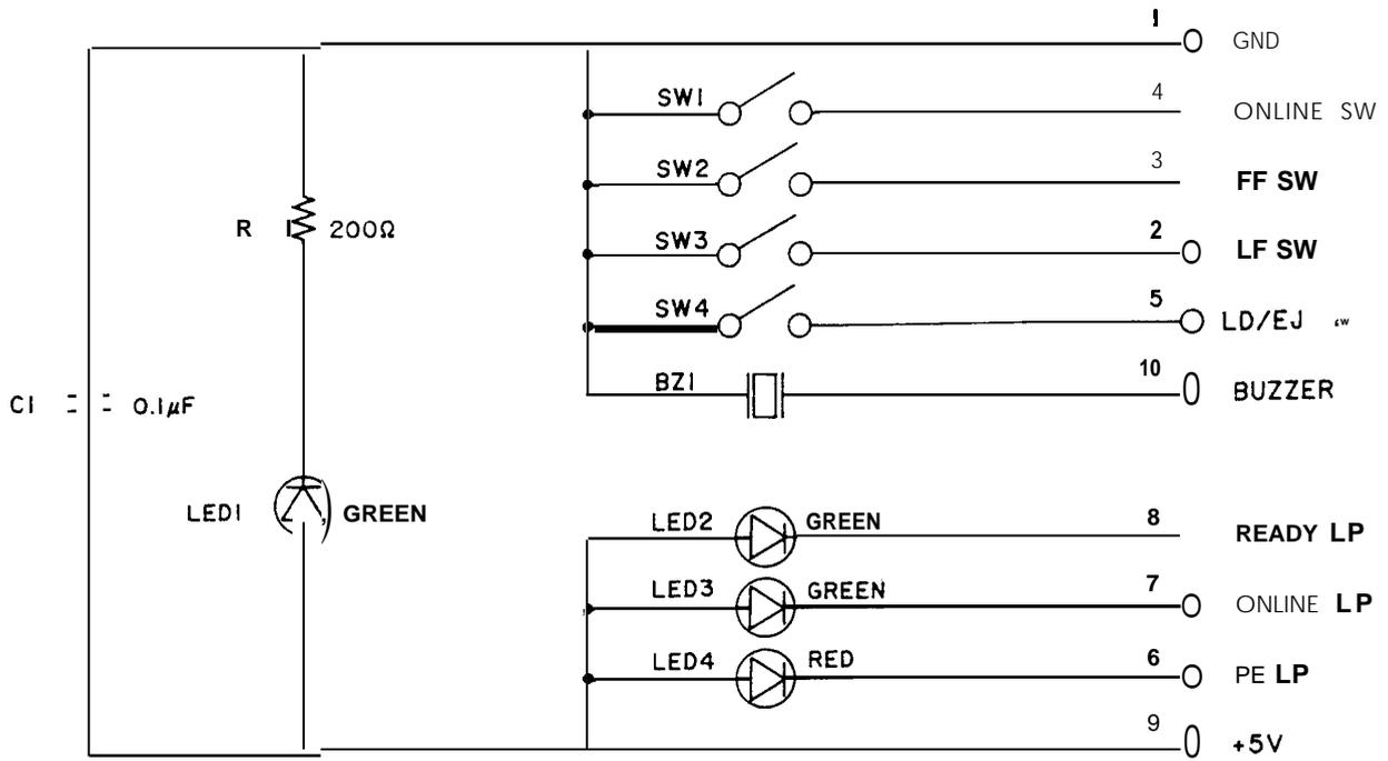
Figure A-1 5. TAPNL-W Board Circuit Diagram
