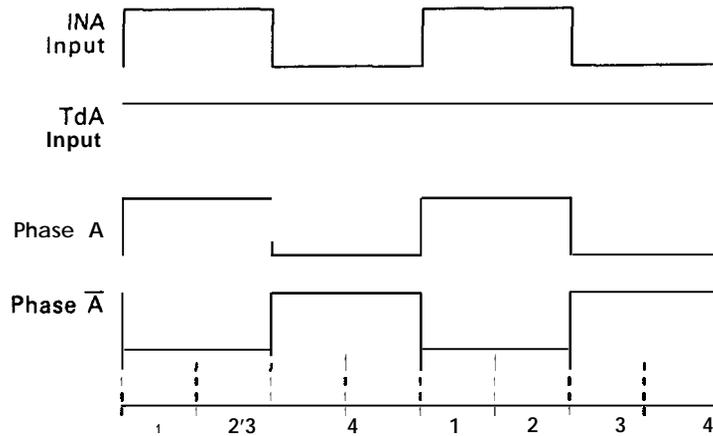
**Figure 2-29. Phase Signal Timing Chart (2-2 Phase)**
