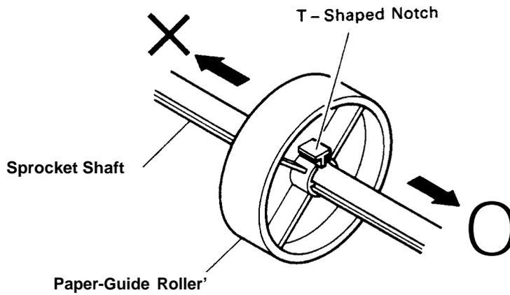
Figure 3-16. Direction of Paper Guide Roller Removal
