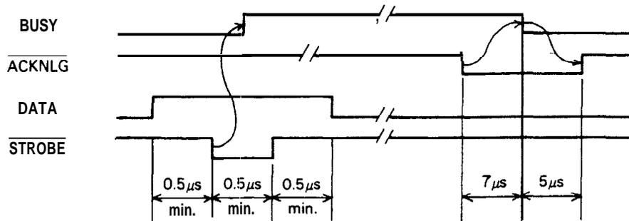
Figure 1-6. Data Transmission Timing
