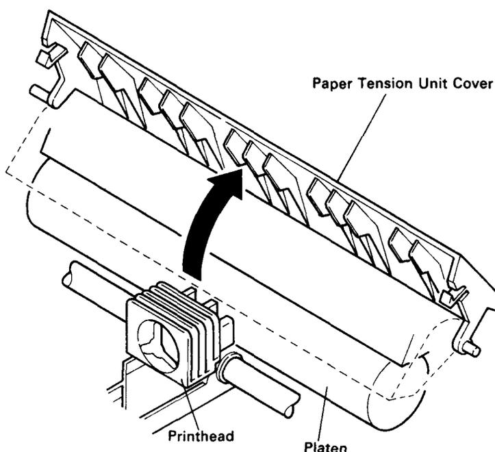
Figure 4-1. Paper Tension Unit Cover
