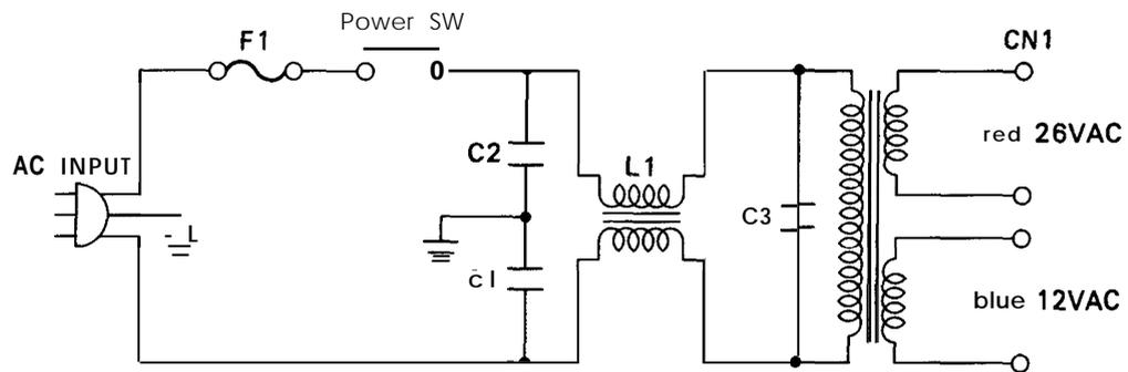
Figure A-1 4. TA Filter Unit Circuit Diagram
