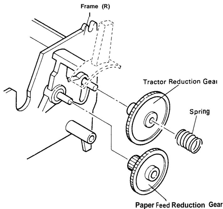
Figure 4-22. Spring and Gear Removal
