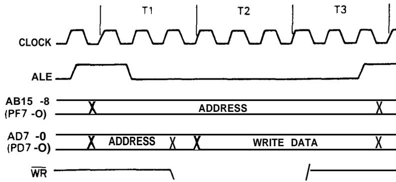
**Figure A-5. Memory Write Timing**
