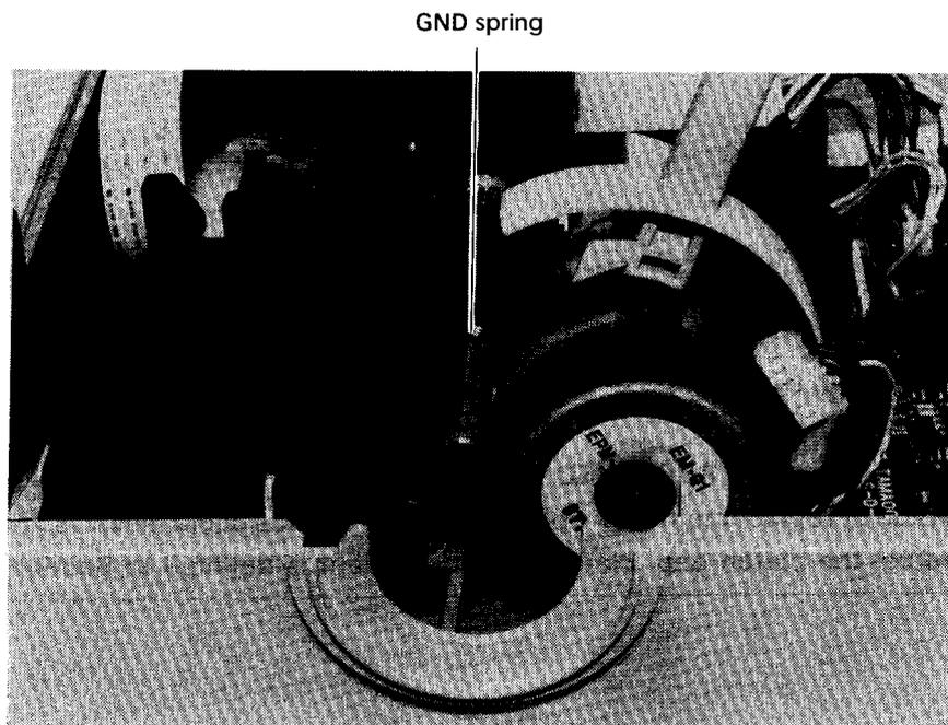
Figure 4-14. GND Spring Removal
