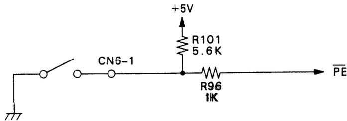
Figure 2-4. Paper-End Sensor Circuit
