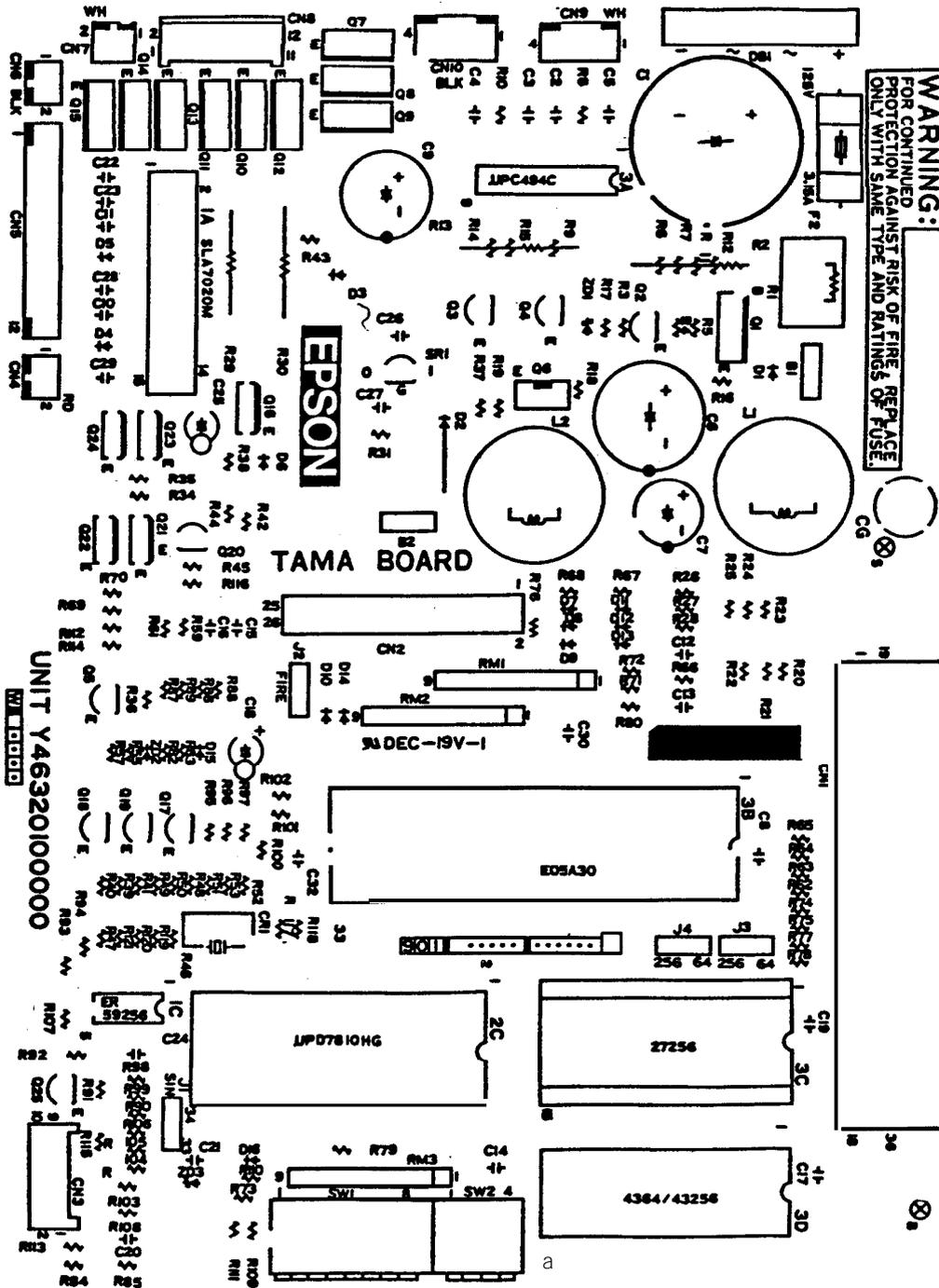
Figure A-1 6. TAMA Board Component Layout
