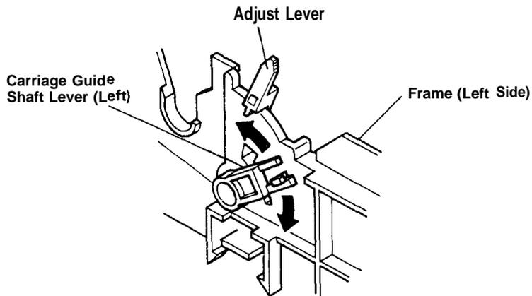
Figure 4-41. Carriage Guide Shaft Lever Movement
