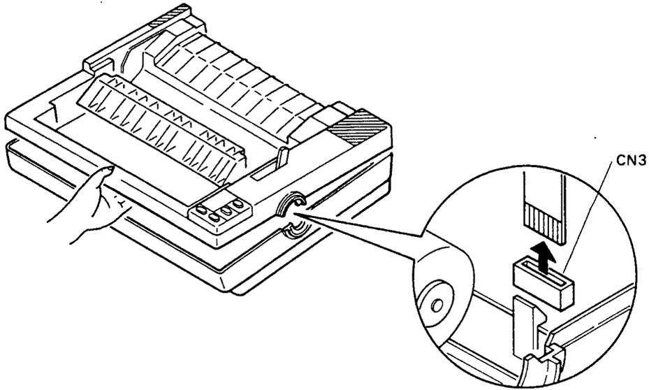
Figure 4-6. Upper Casing Removal -2
