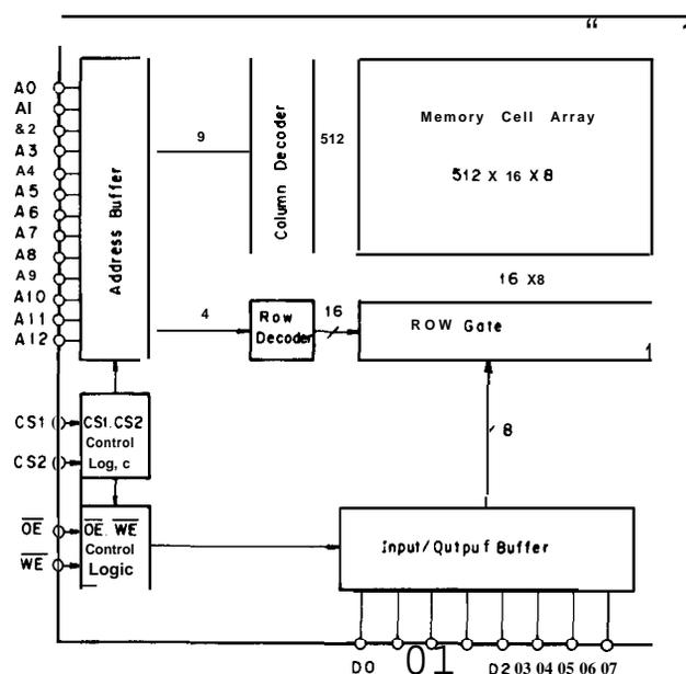
Figure A-8. 2064C SRAM Block Diagram
