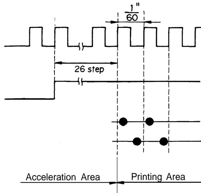
Figure 2-37. Printing Area and Printing Timing
