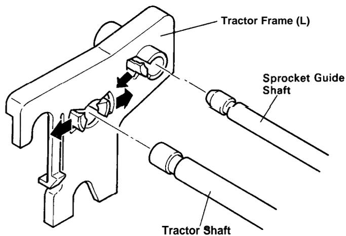
Figure 4-36. Removal of Tractor Frame L
