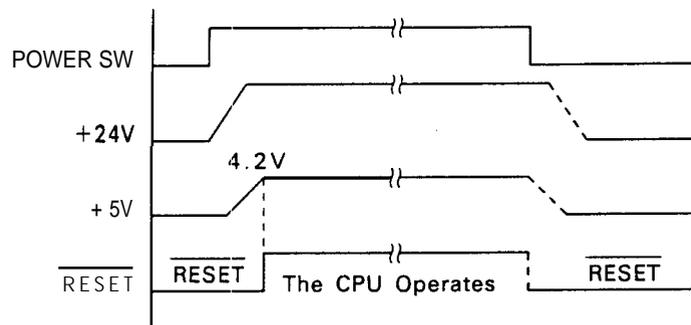
Figure 2-23. RESET Output
