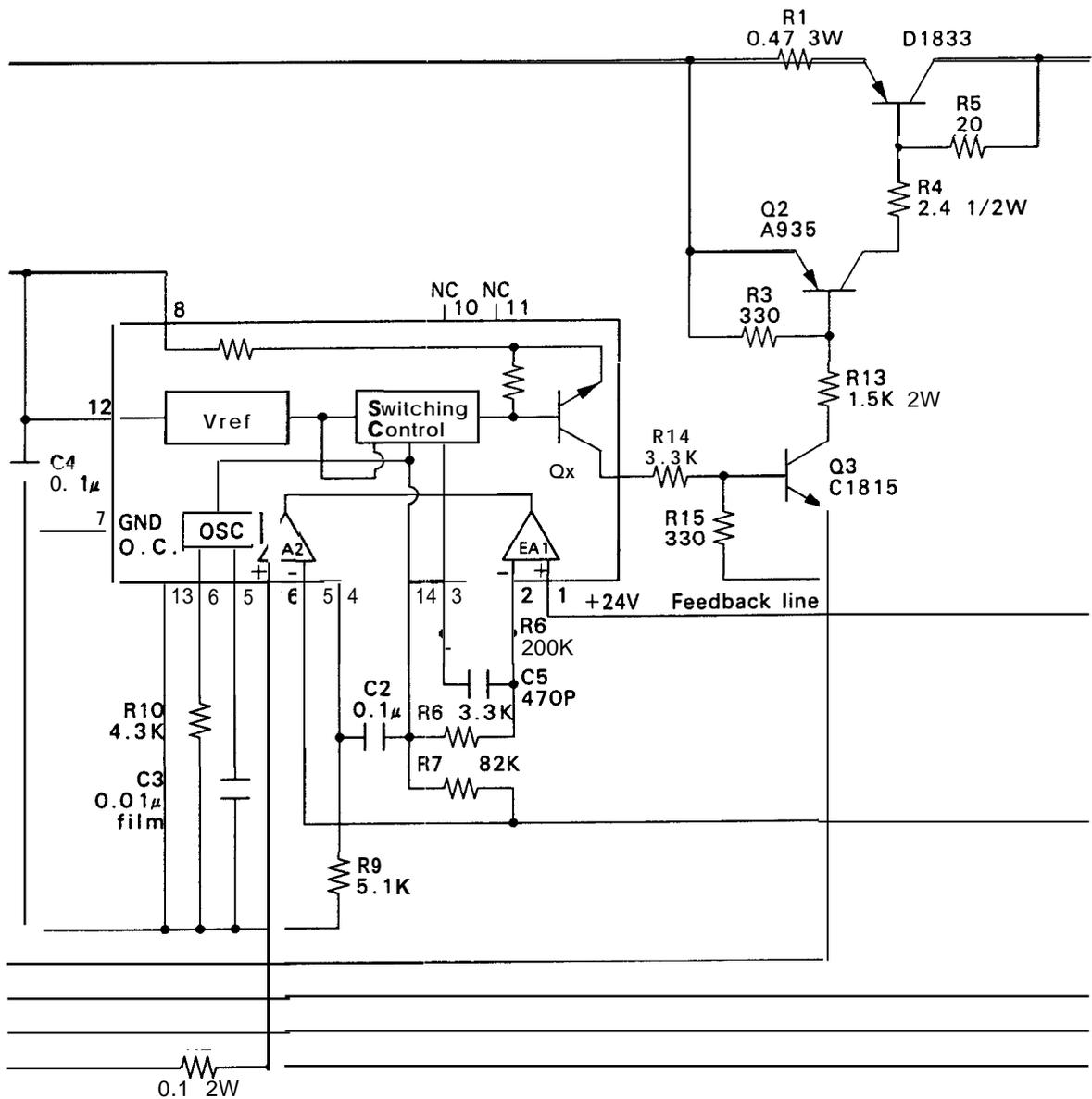
Figure 2-16. +24VDC Switching Regulator Circuit
