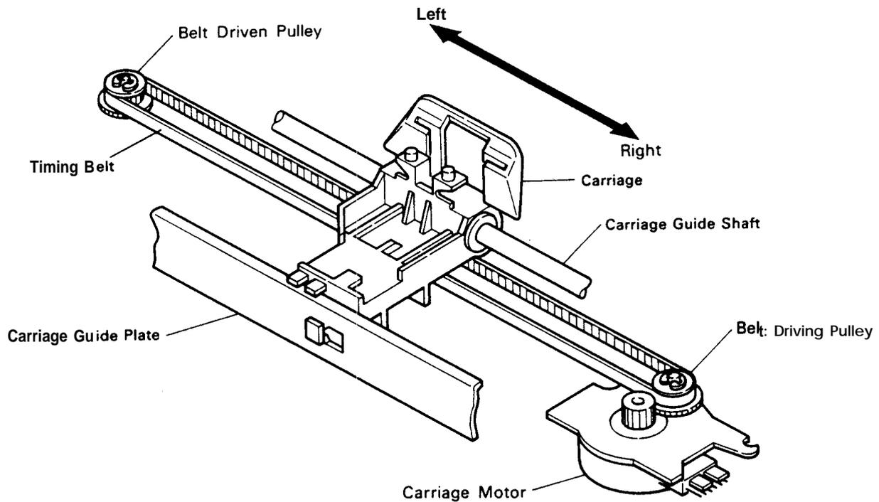
Figure 2-24. Carriage Mechanism
