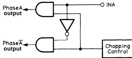
**Figure 2-28. Phase Data Input Circuit (2-2 Phase)**
