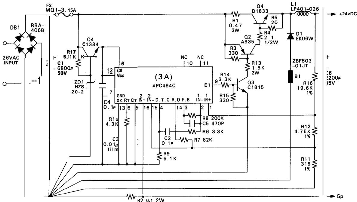
Figure 2-14. +24V DC Power Supply Circuit
