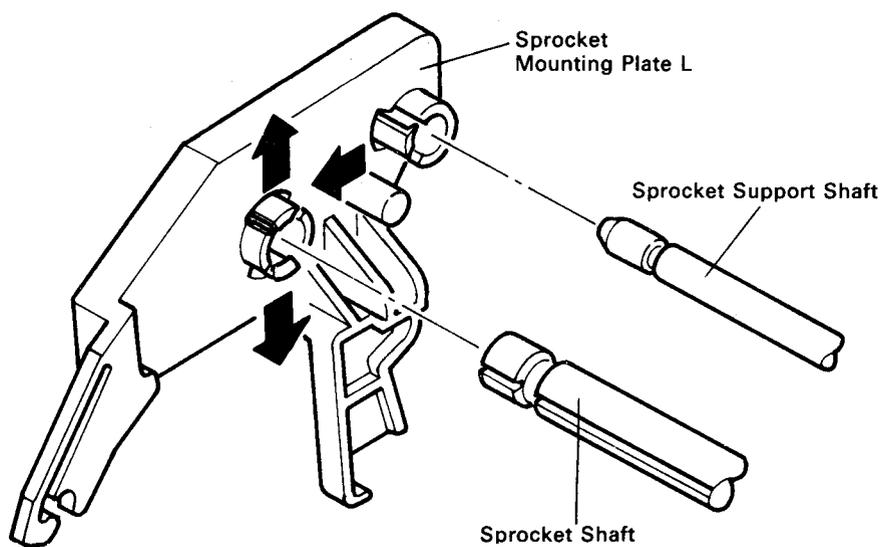
Figure 3-14. Removal of Sprocket Mounting Plate L
