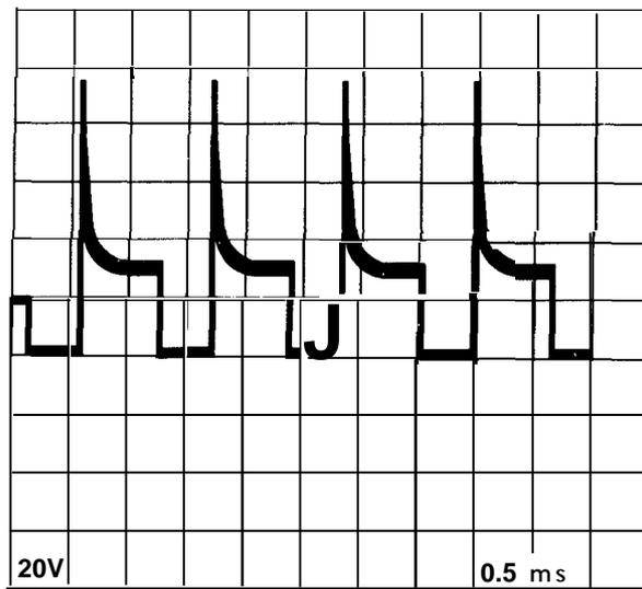
Figure 2-45. Printhead Driving Waveforms
