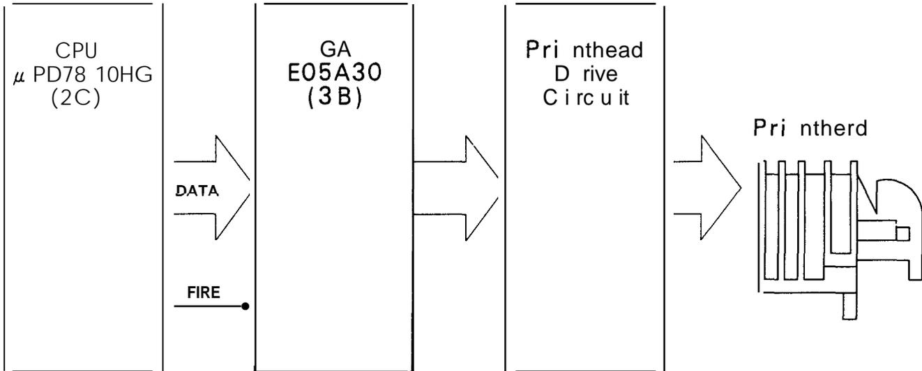
Figure 2-43. Printhead Drive Circuit Block Diagram
