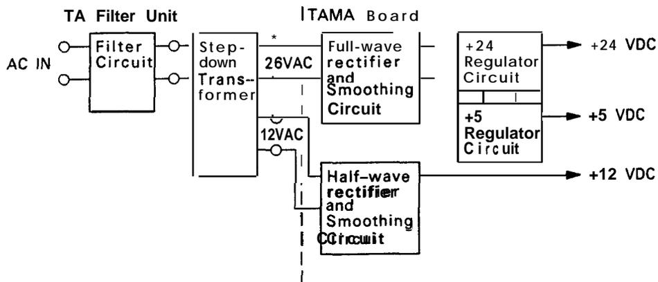
Figure 2-11. Power Supply Circuit Block Diagram
