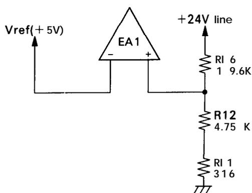
Figure 2-17. Voltage Feedback Circuit
