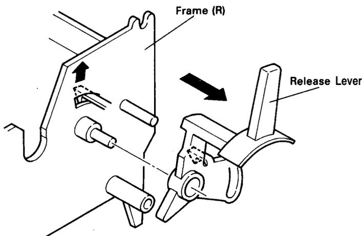
Figure 4-23. Removal of The Release Lever
