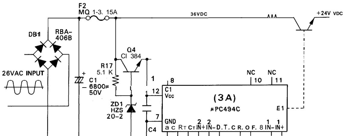
Figure 2-15. Rectifier and Smoothing Circuit
