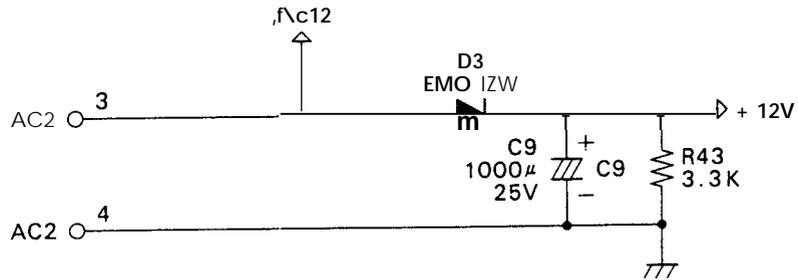
Figure 2-13. + 12V DC Power Supply Circuit
