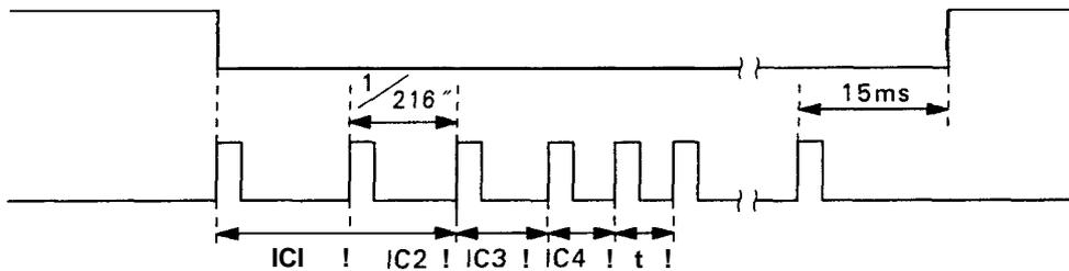
Figure 2-41. Paper-Feed Motor Drive Timing Chart
