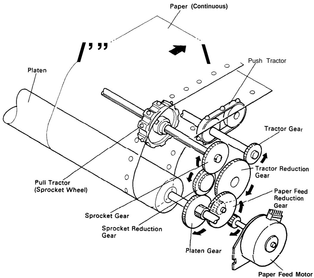
Figure 3-12. Push-Pull Feed Operation
