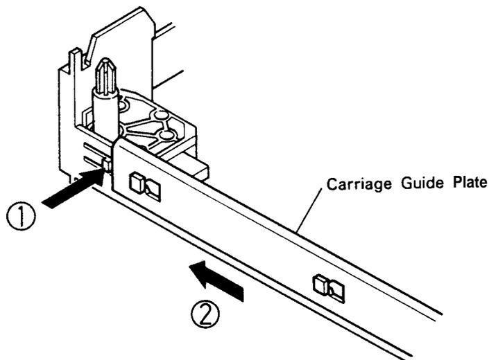
Figure 4-30. Removal of Carriage Guide Plate
