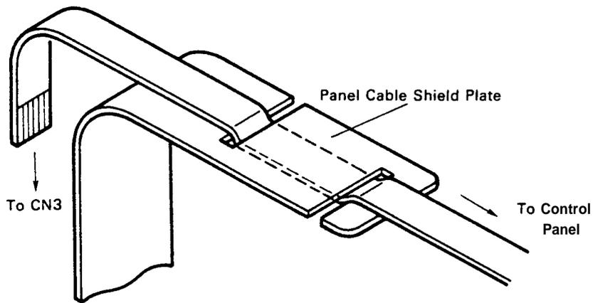
Figure 4-7. Control Panel FFC
