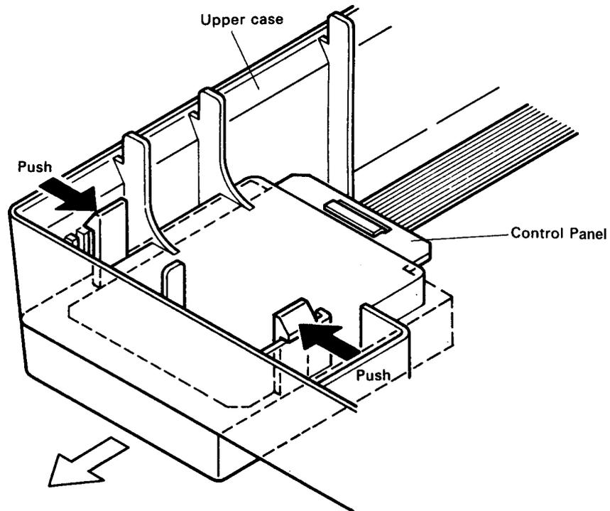
Figure 4-8. Control Panel Removal
