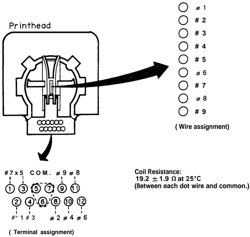
Figure 5-1. Printhead Resistance
