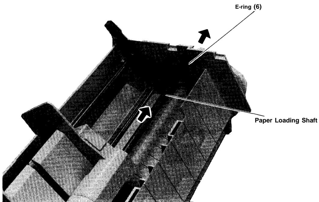
Figure 3-6. Paper Loading Roller Shaft Removal
