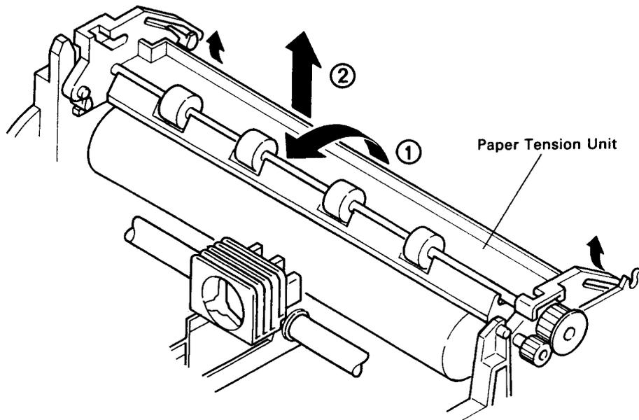
Figure 4-13. Paper Tension Unit Removal
