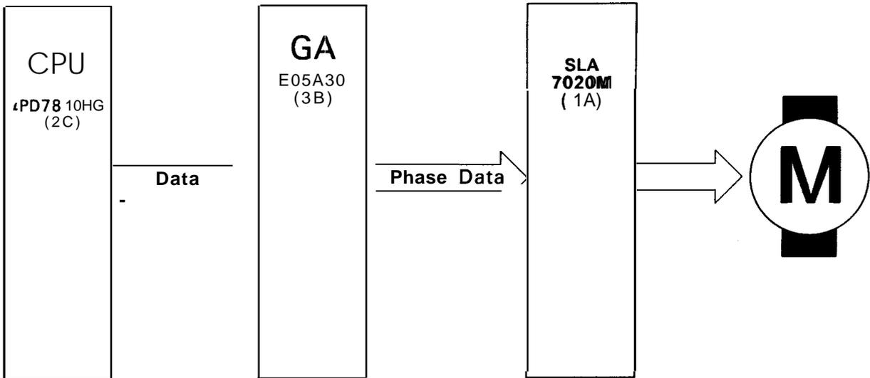
Figure 2-25. Carriage Drive Circuit Block Diagram
