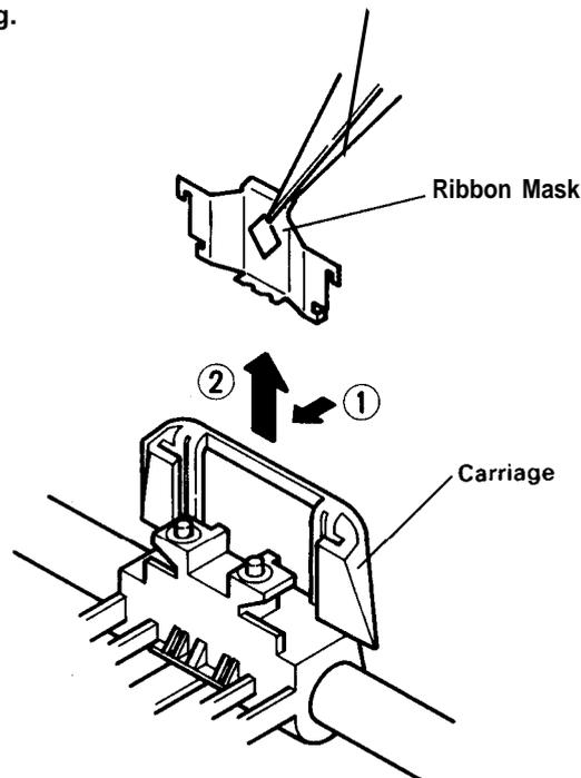
Figure 4-39. Removal of Ribbon Mask
