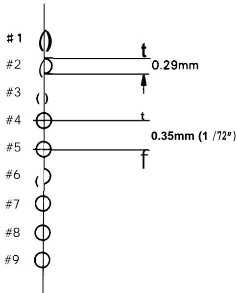
Figure 1-2. Pin Configuration
