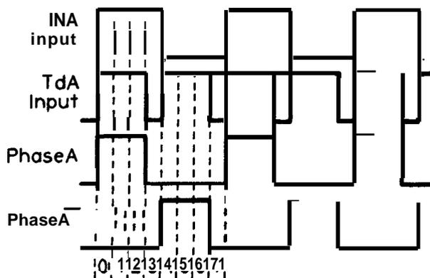
Figure 2-31. Phase Signal Timing Chart (I-2 Phase)
