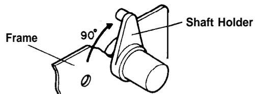
Figure 3-8. Shaft Holder Removal
