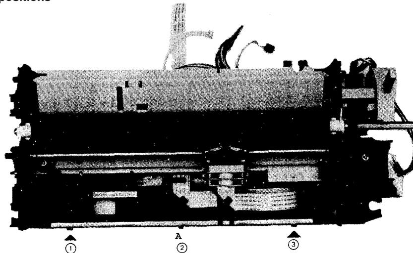
Figure 4-42. Platen Gap Adjustment Position
