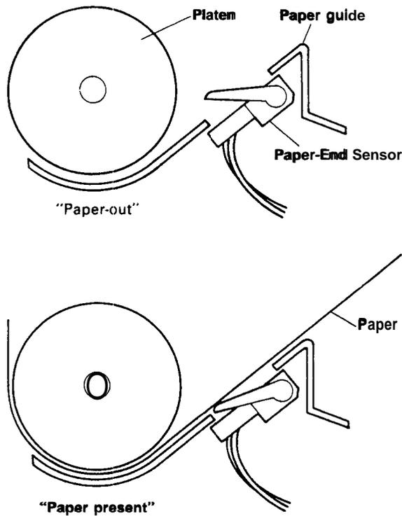
Figure 2-3. Paper-End Sensor Mechanism
