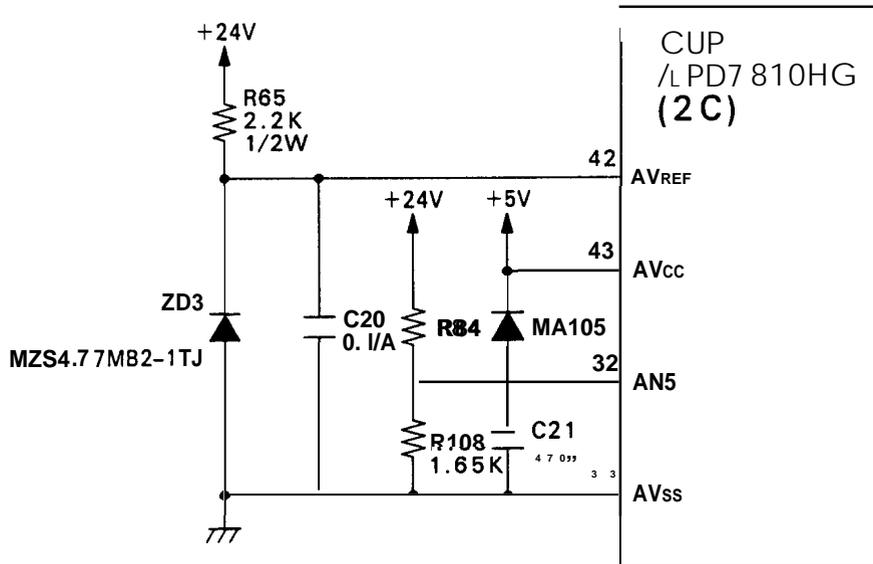
Figure 2-47. A/D Converter (+24 VDC Line Monitor) Circuit
