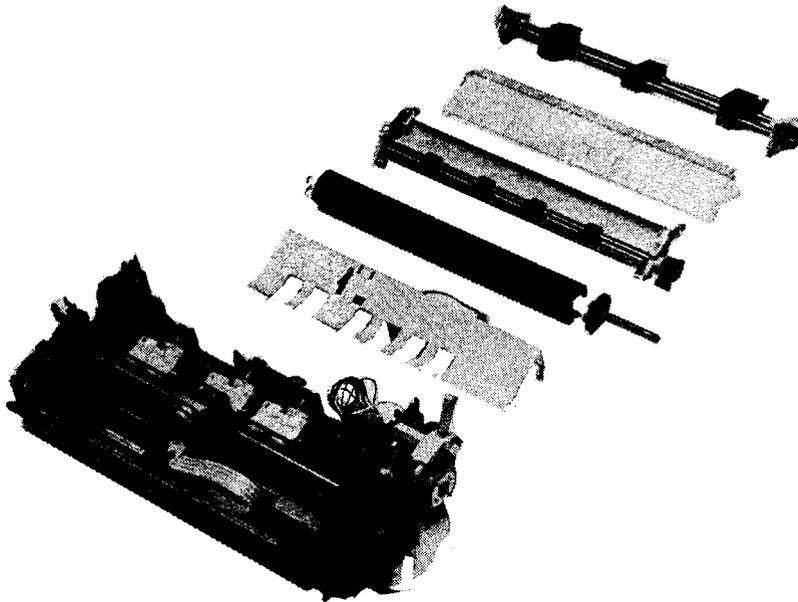
Figure 4-11. Printer Mechanism Removal
