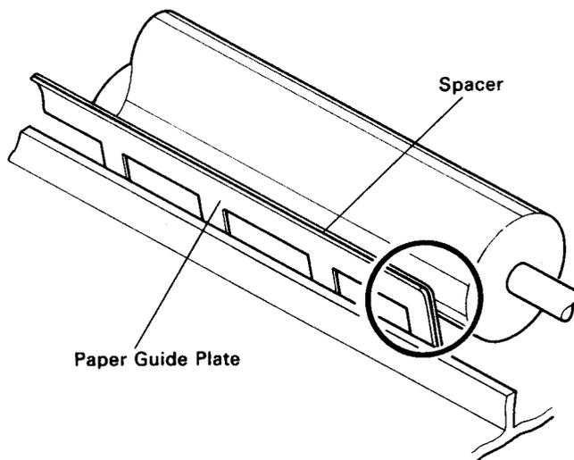
Figure 4-20. Mounting Direction for Paper Guide Plate
