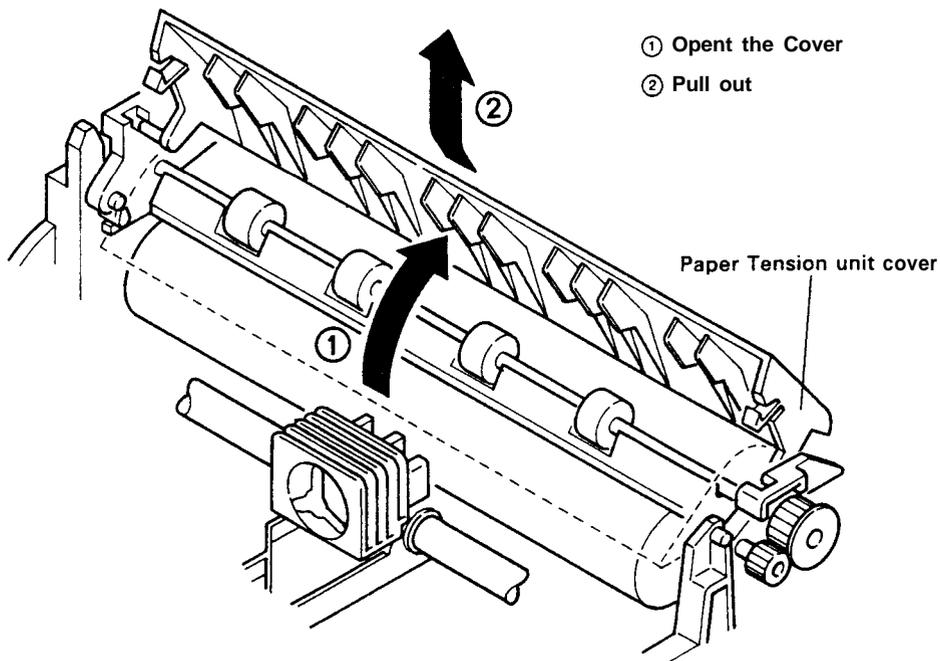
Figure 4-12. Removal of Paper Tension Unit Cover
