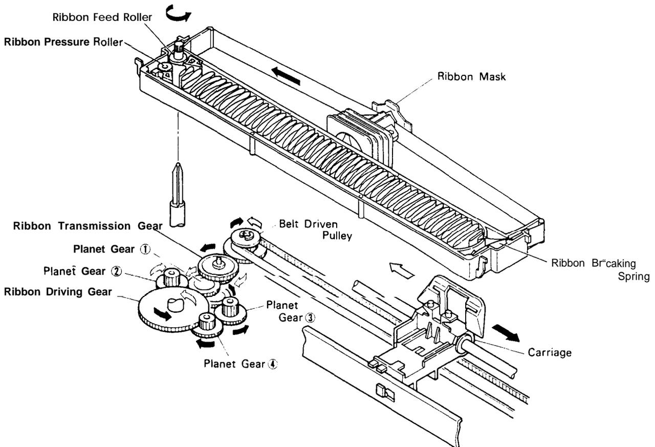
**Figure 2-51. Ribbon-Feed Mechanism**
