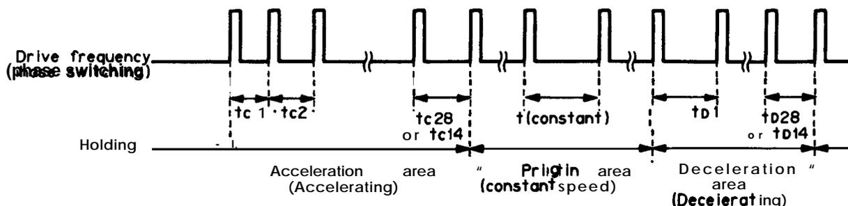
Figure 2-35. Carriage Motor Control
