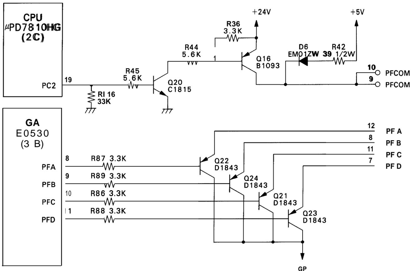
Figure 2-40. Paper-Feed Motor Drive Circuit
