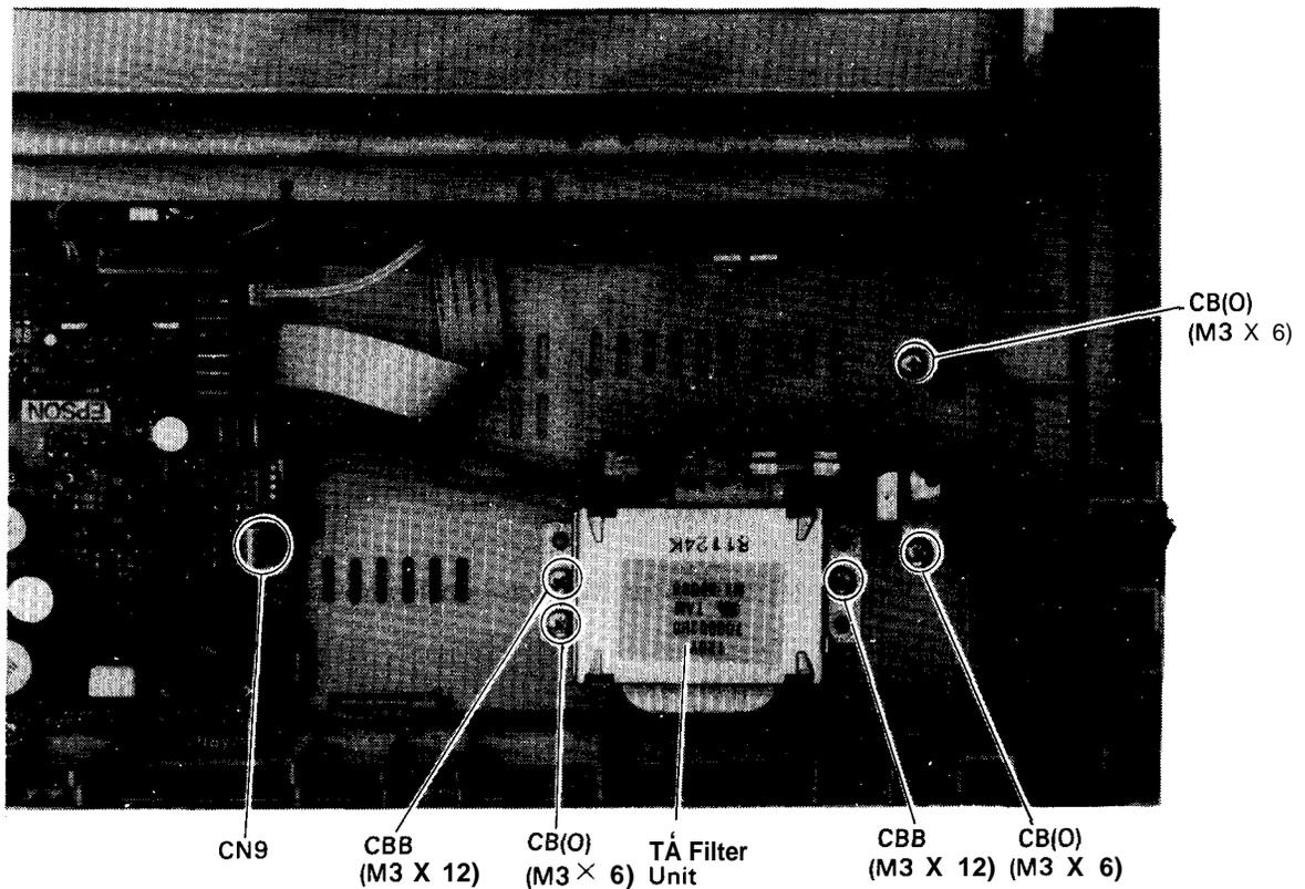
Figure 4-10. TA Filter Unit Removal
