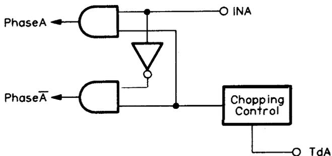
Figure 2-30. Phase Data Input Circuit (I-2 Phase)
