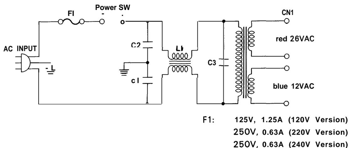
Figure 2-12. Transformer Circuit
