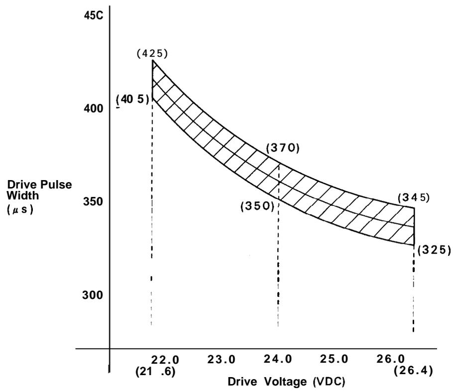
Figure 2-48. Relationship between Head Driver Voltage and Print Driving Pulse Width
