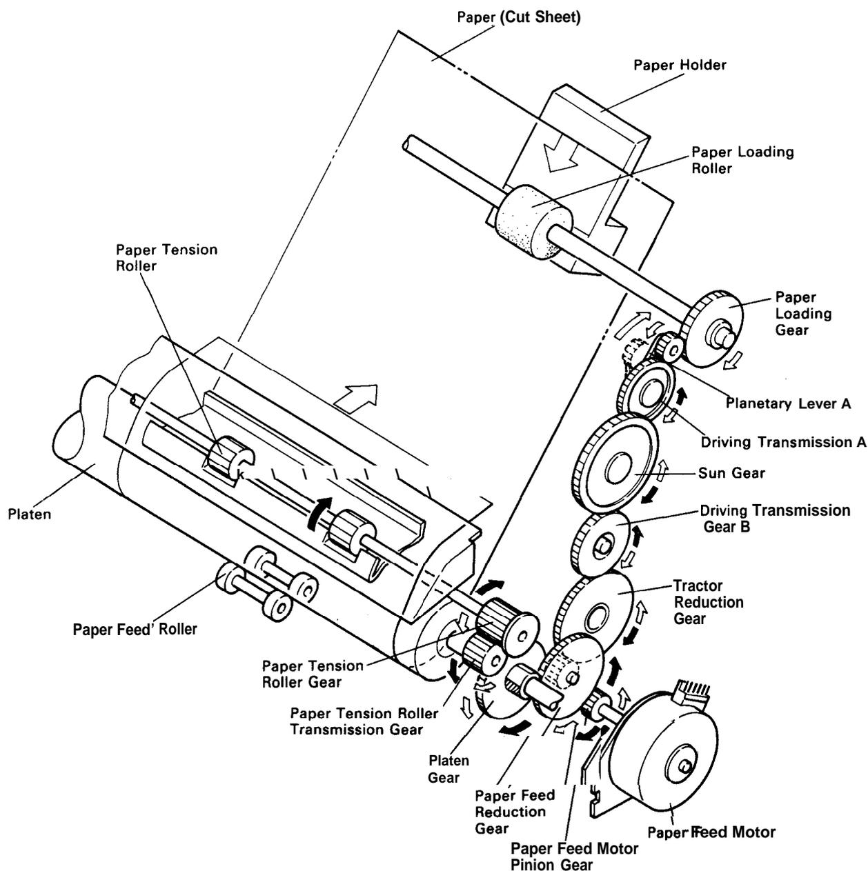
Figure 3-4. Cut Sheet Feeder Operation
