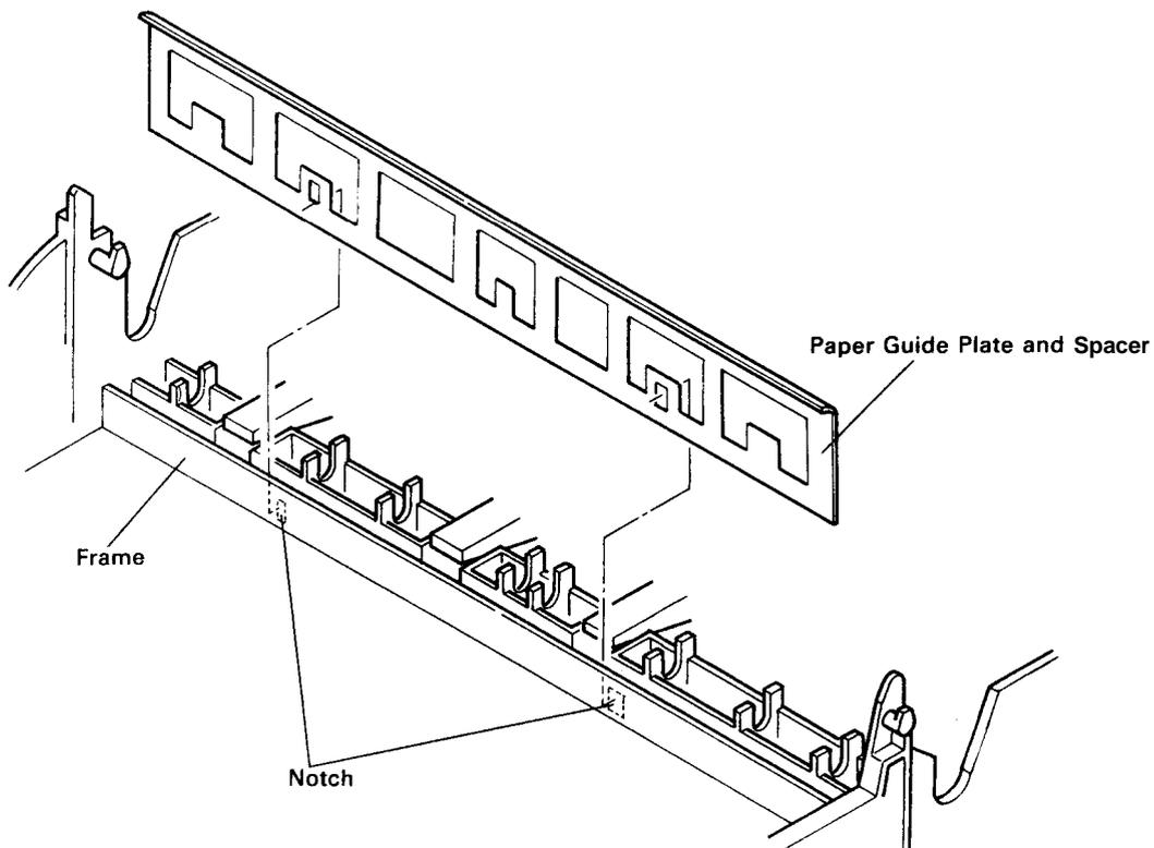
Figure 4-19. Removal of Paper Guide Plate
