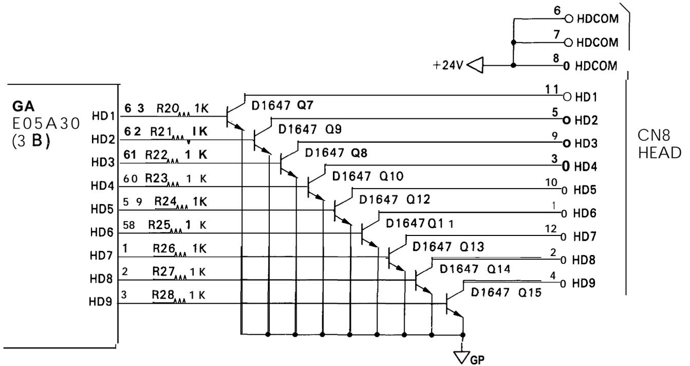
Figure 2-44. Printhead Drive Circuit
