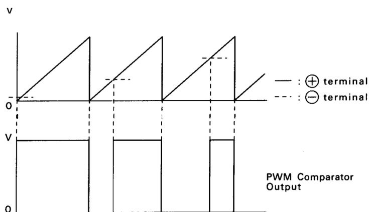
Figure 2-19. output Transistor Drive Waveform
