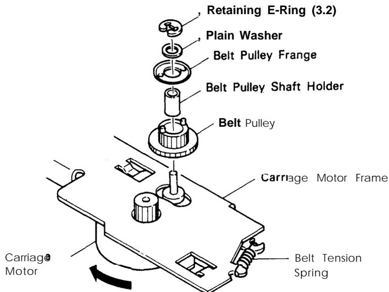
Figure 4-33. Removal of Carriage Motor
