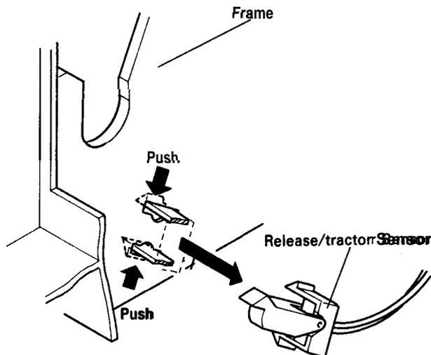
Figure 4-24. Removal of Release/Tractor Sensor
