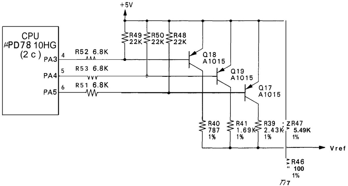
Figure 2-32. Reference Voltage Generation Circuit
