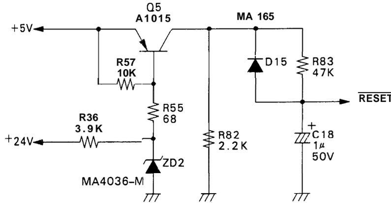
Figure 2-22. Reset Circuit
