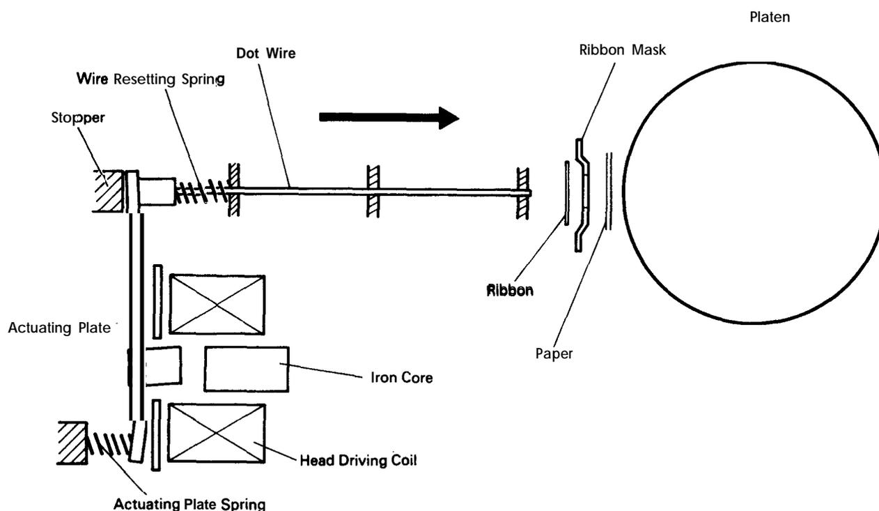
Figure 2-42. Printhead Printing Operation
