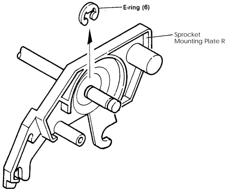
Figure 3-15. Removal of Sprocket Mounting Plate.
