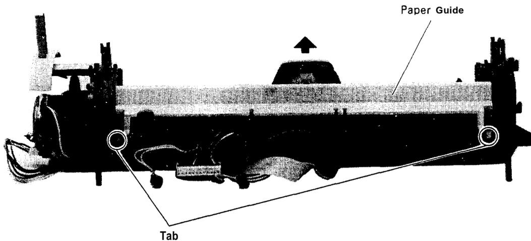
Figure 4-16. Rear View of Printer Mechanism
