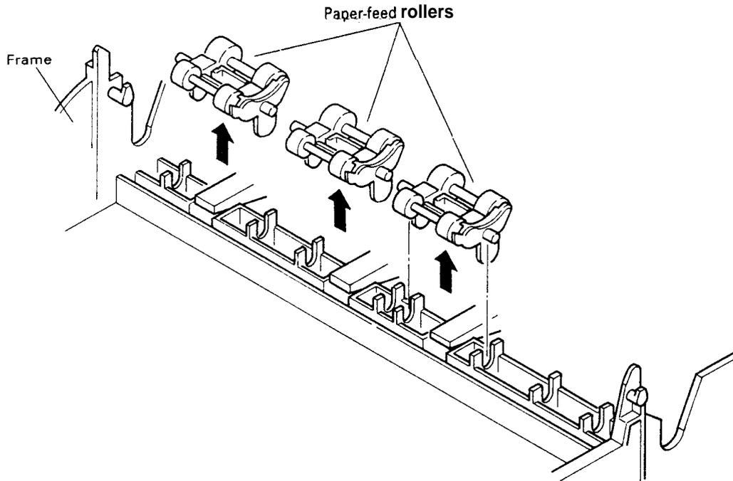
Figure 4-18. Removal of Paper Feed Rollers
