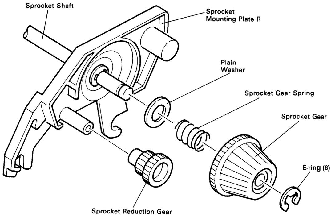
Figure 3-13. Removal of Sprocket's Intermediate Gear and Related Parts
