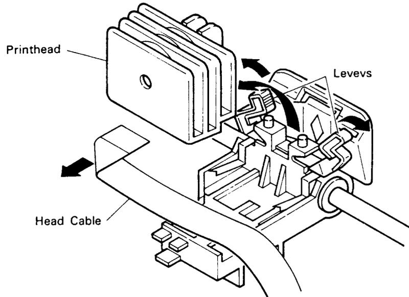
Figure 4-2. Printhead Removal
