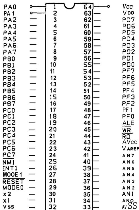
Figure A-1.  $\mu$ PD7810HG Pin Diagram
