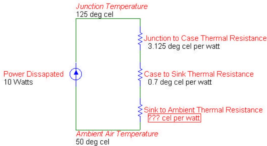
Fig A - Schematic Diagram for Power Dissipation of TIP32C pass device.
