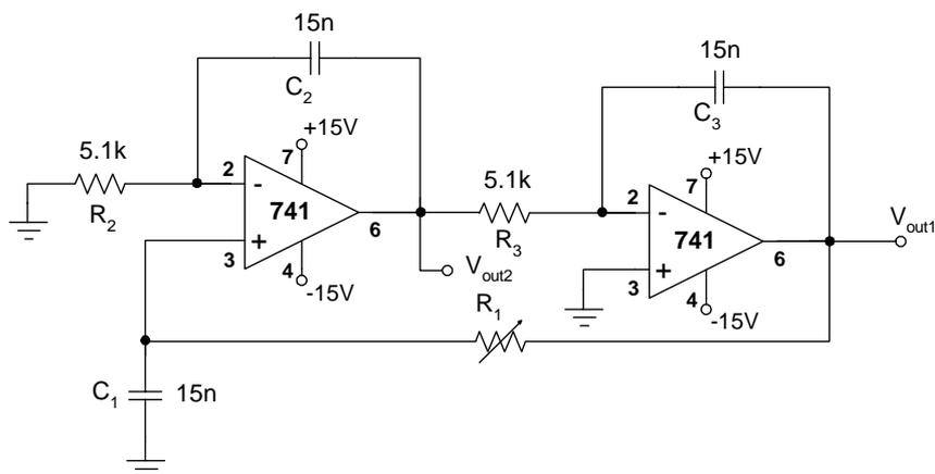
$$f_0 = 1/2\pi\sqrt{C_2 C_3 R_2 R_3}$$
