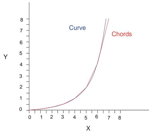
Let X represent an input voltage from a sensor with a non linear output.
