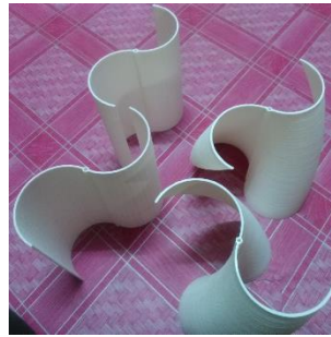
Figure 3.8: Separation part of conventional and helical blade rotors
