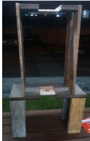
Figure 3.17: Complete structure of the VAWT tower
