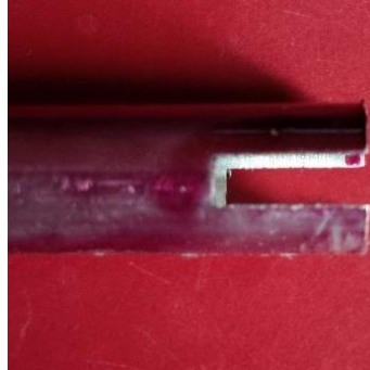
Figure 3.11: Slots at the end of rods with diameter 0.75 cm hollow
