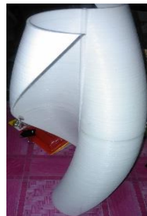
Figure 3.9: Helical blade rotor that had been attached
