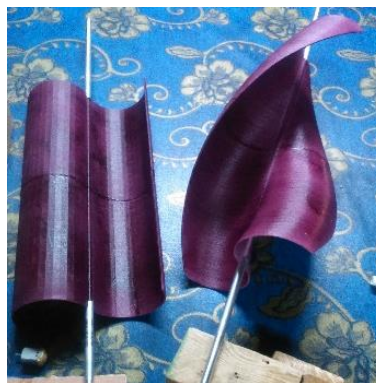
Figure 3.12: The combination of blade rotors and shaft
