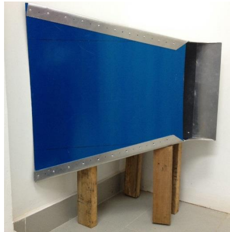
Figure 3.14: Complete structure of the wind concentrator.
