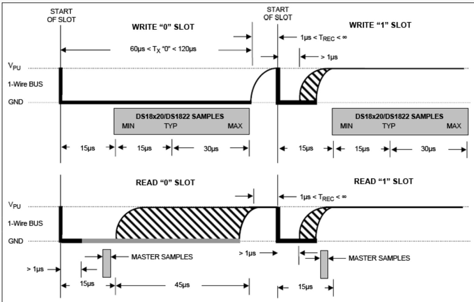
Figure 3. Write and read time slots.
