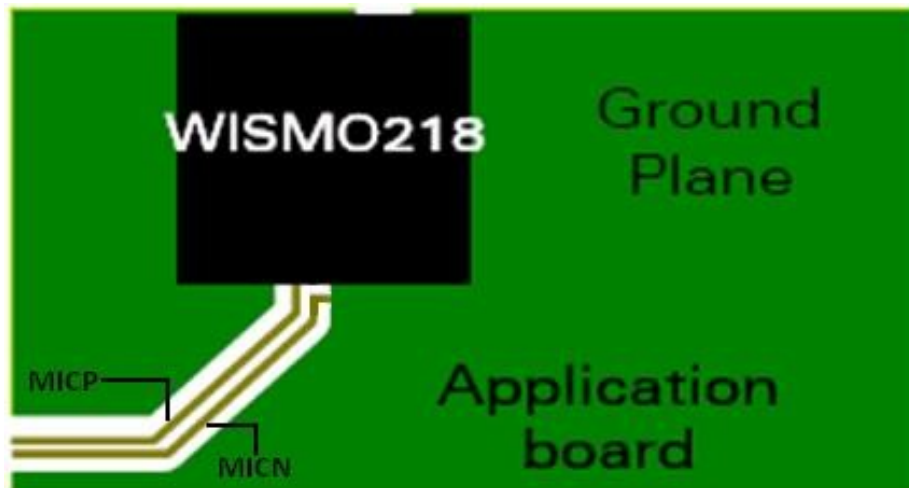
Figure 24. Single-Ended Audio Connection
