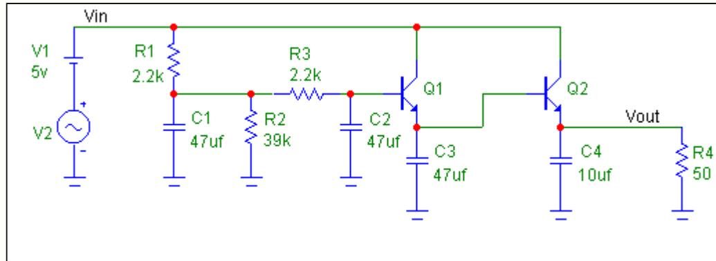
With the values shown, this method provides good attenuation from 50 Hz to 100 MHz. The attenuation floor between 100 Hz and 10 KHz is determined by the impedance of transistor Q2, which will vary from one transistor to the next.
