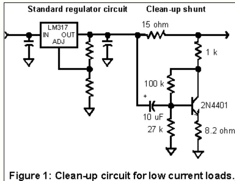
Figure 1: Clean-up circuit for low current loads.
