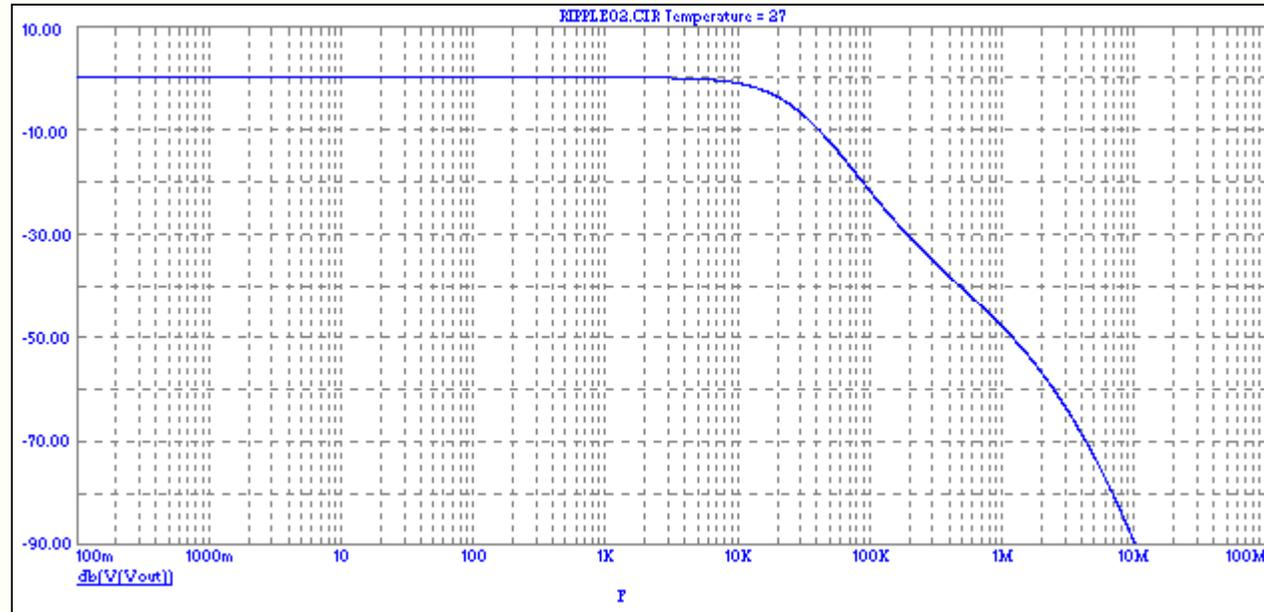
Adding more RC sections to the ripple filter (RIC1) can increase the notch depth, but have little effect above 1 KHz.
