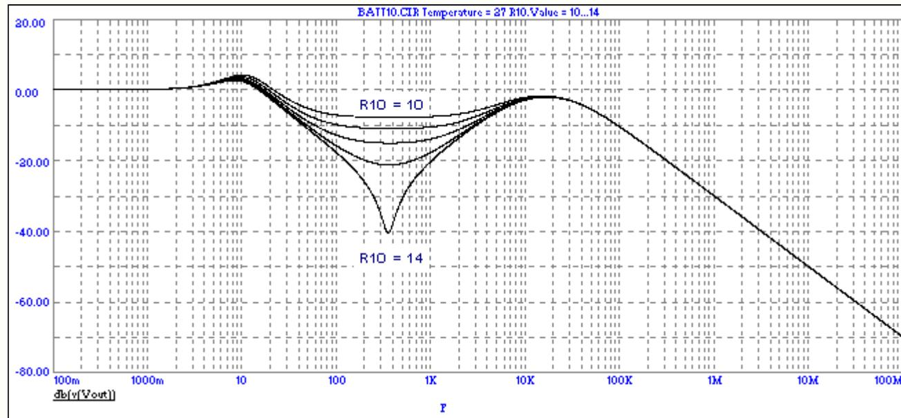
The null has moved down from about 8 KHz to 130 Hz and shows less attenuation than the single transistor version in Figure 1. In addition, the op amp now contributes its own broadband noise to the output.
