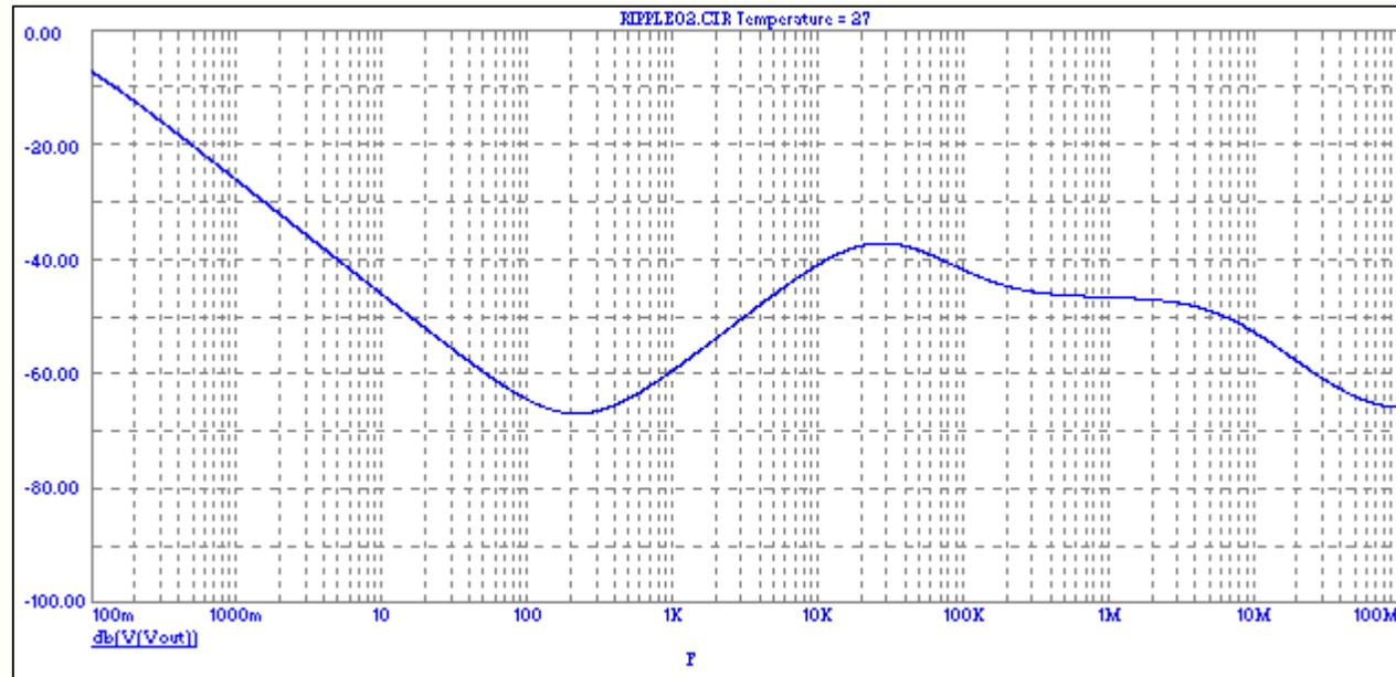
The MAX495 is specified at 25 nV/sqrt(Hz), or approximately 2.5 uV rms from 1 to 10 KHz. This is similar to the LM723 [1]. The plot below shows how the noise appears at the output of the regulator:
