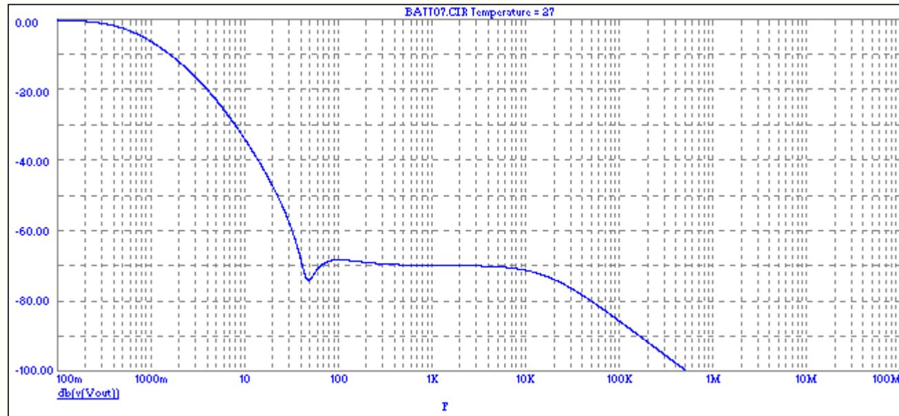
The performance above 10 KHz is determined by the ESR of the filter capacitors and the circuit layout. In order to improve the performance at higher frequencies, multiple ceramic capacitors can be added in parallel with the electrolytic. These are usually provided by the bypass capacitors
