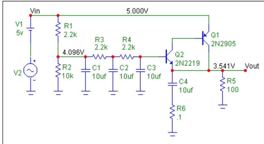
The attenuation is similar to the Darlington. The attenuation floor between 100 Hz and 100 KHz is determined by the loop gain, which is device-dependent. The response above 100 KHz is largely determined by the ESR of the output capacitor C4.
