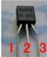
TO92 package's pin arrangement
