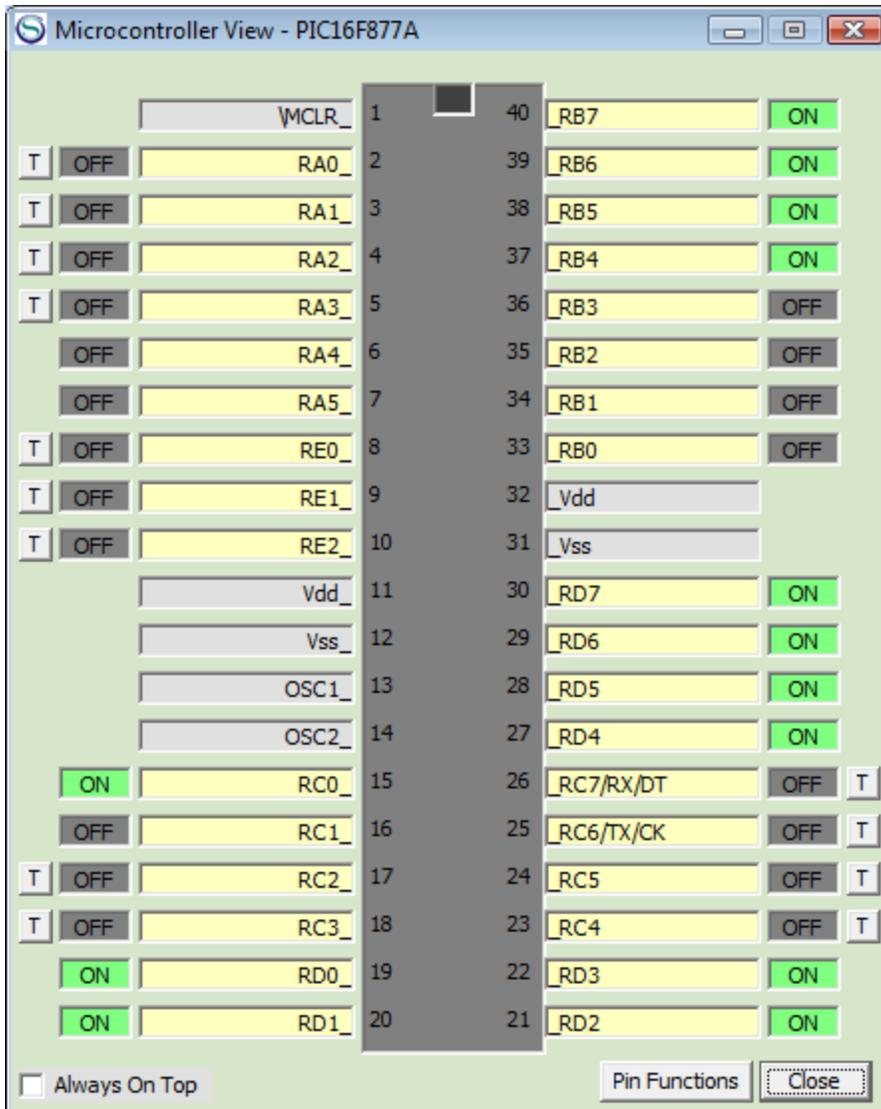
RB seems to be data out. RD7, 6, 5 are toggled low momentarily in that sequence, followed by RC1 going high (toggled high then low). Toggle times seem to be 5ms low, then 5ms before next pin is toggled. RC1 is reversed. (10ms cycle time per character). This is assuming 4Mhz clock. If clock is higher, like 8Mhz, then times will be 1/2 of those listed, etc...
