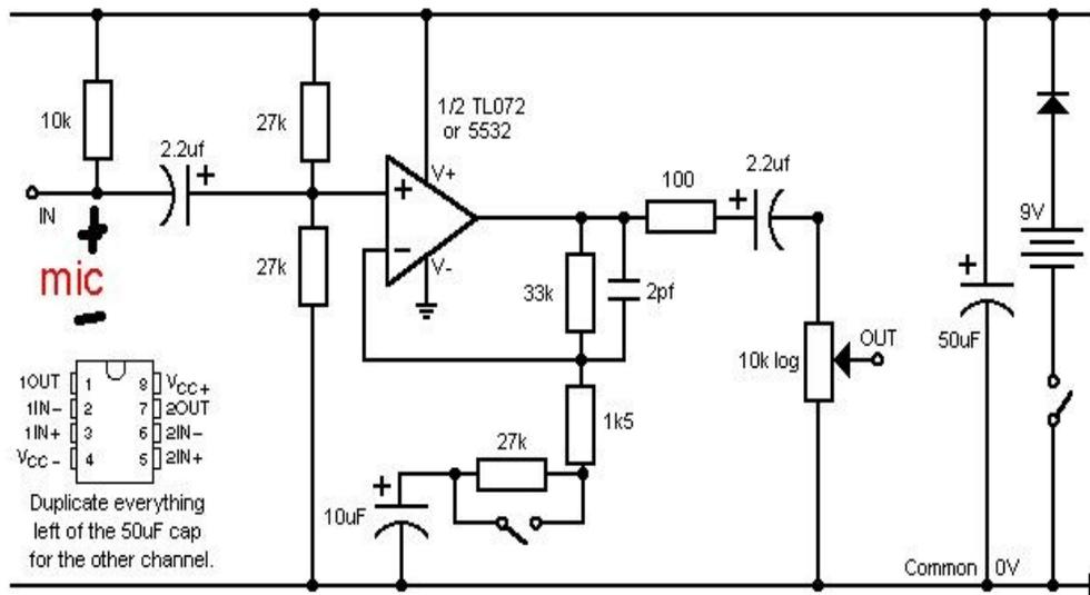
*Schematic Of One Channel - Single Rail Version (Slight Difference From Text)*
