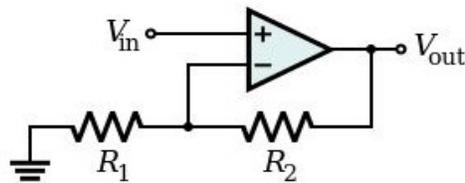
An op-amp connected in the non-inverting amplifier configuration
