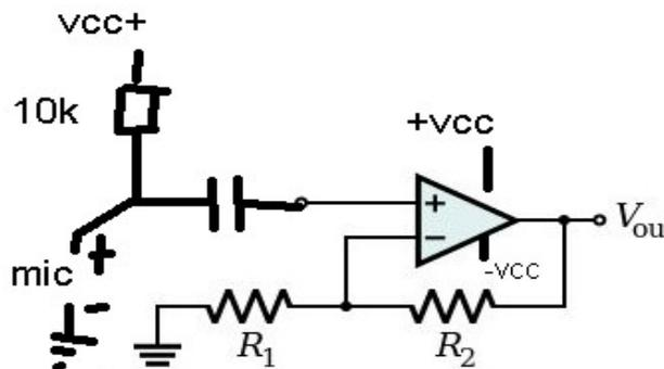
An op-amp connected in the non-inverting amplifier configuration
